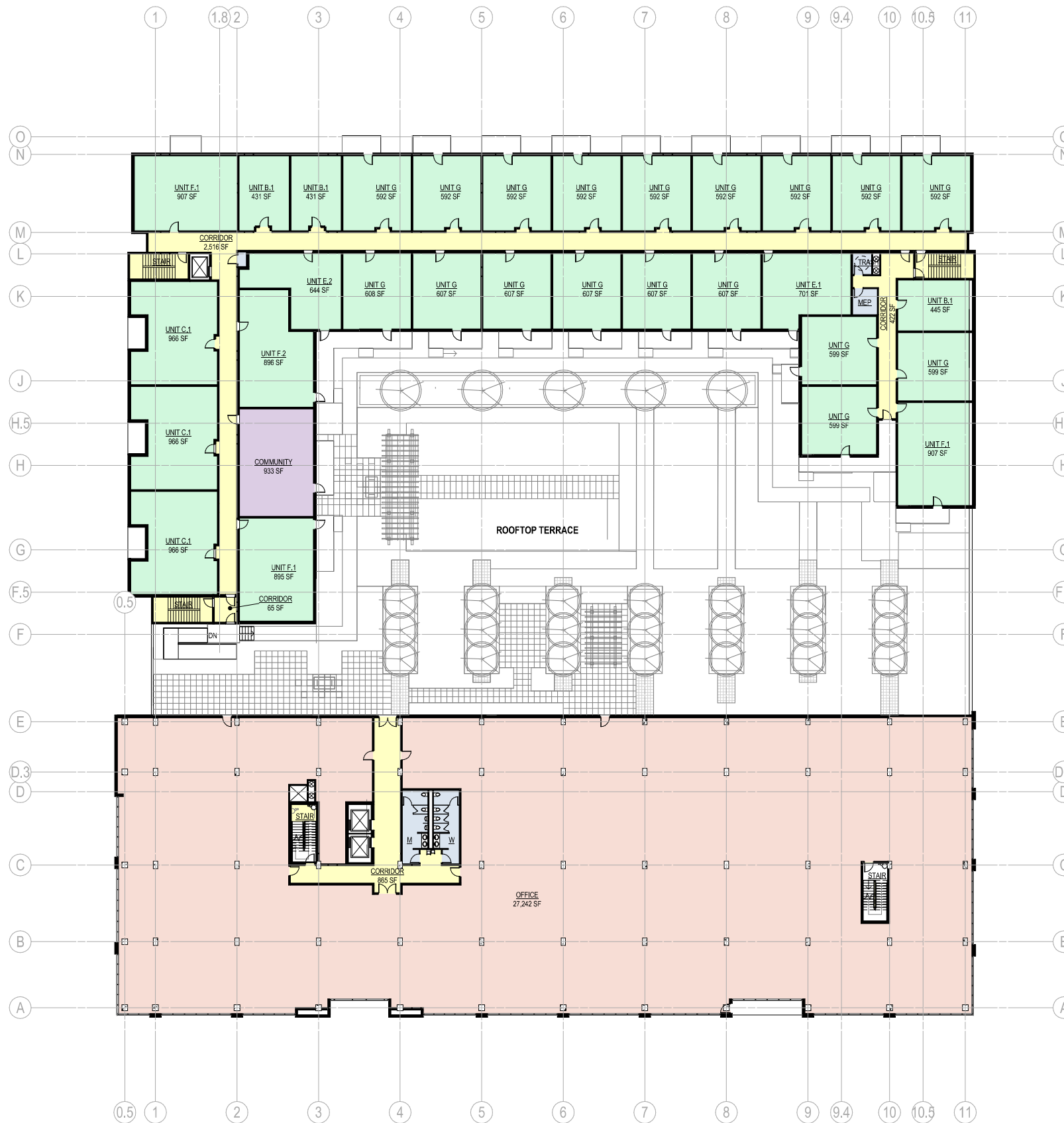
1 LEVEL 03 & LEVEL N-04 FLOOR PLAN 1" = 20'-0"
