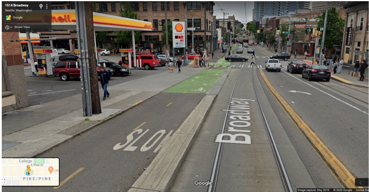
Figure B.4-9 Seattle, WA – Cycletrack is at street level with curbed protection
