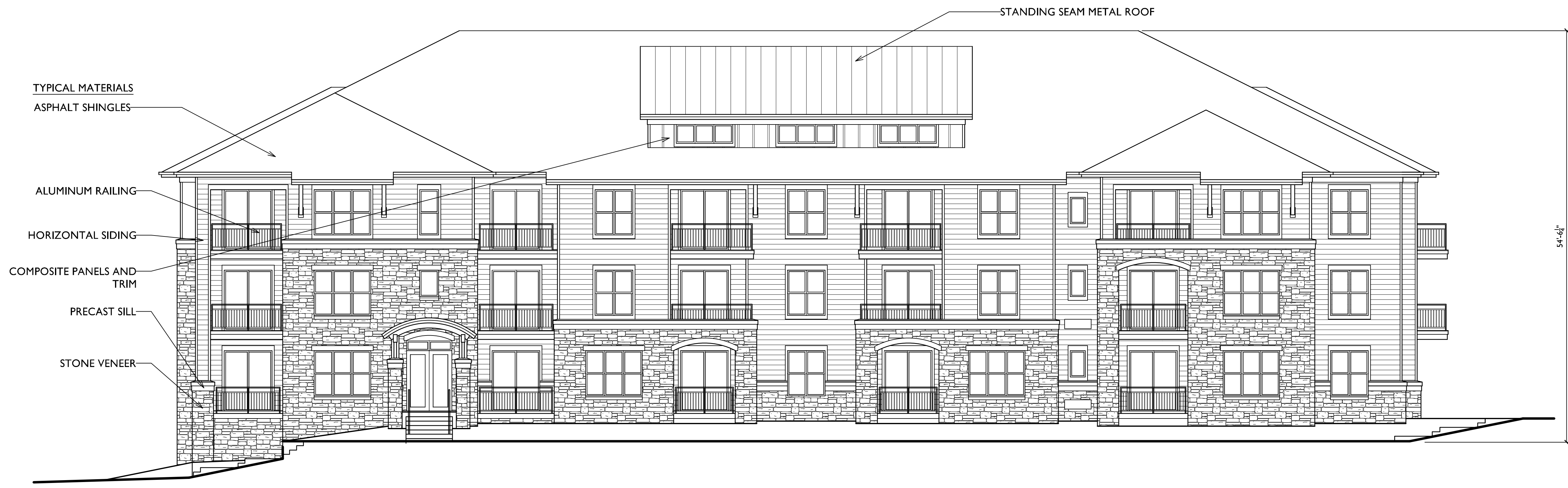
1 33 SOUTH ELEVATION - BUILDING 5 SCALE: 1/8"=1'-0"
