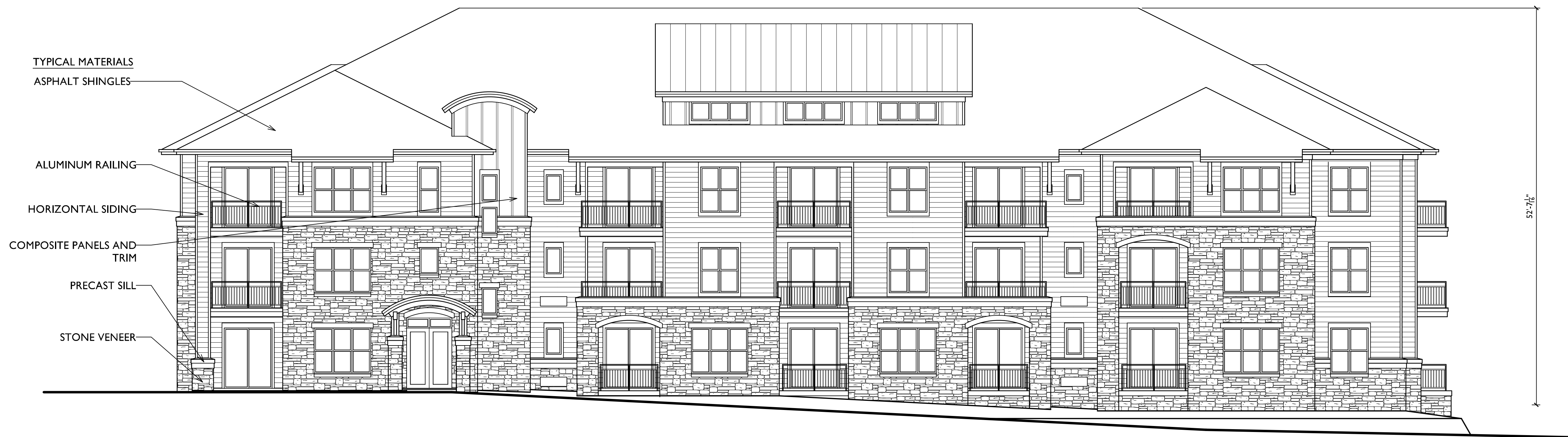
2 NORTH ELEVATION - BUILDING 10 SCALE: 1/8"=1'-0"
