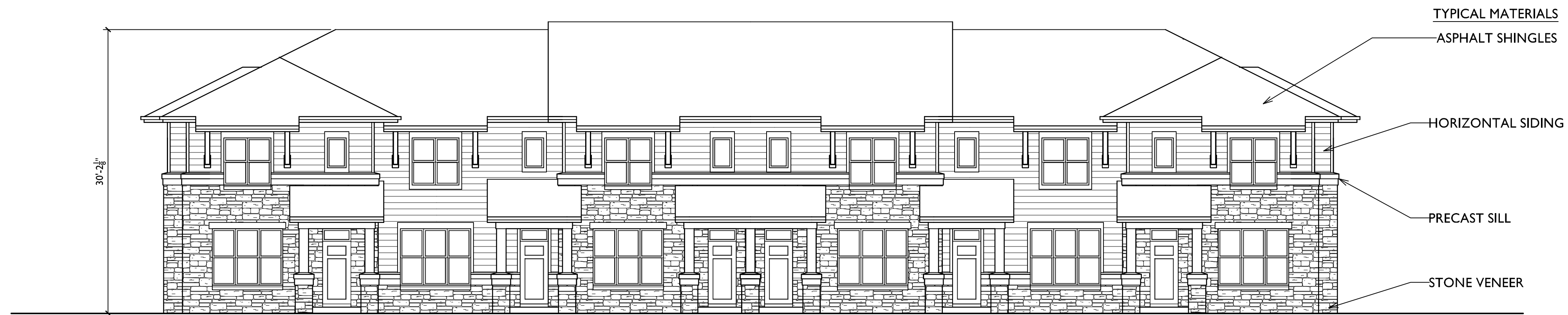
1 EAST ELEVATION - BUILDING 8 SCALE: 1/8"=1'-0"
