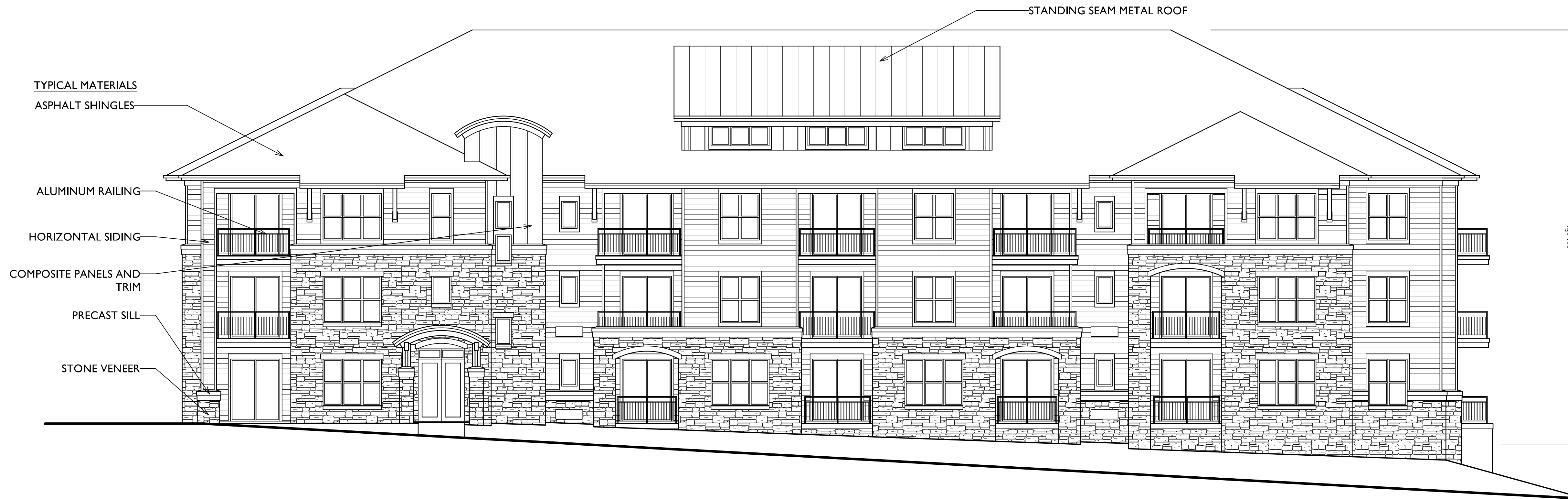
1 32 NORTH ELEVATION - BUILDING 5 SCALE: 1/8"=1'-0"
