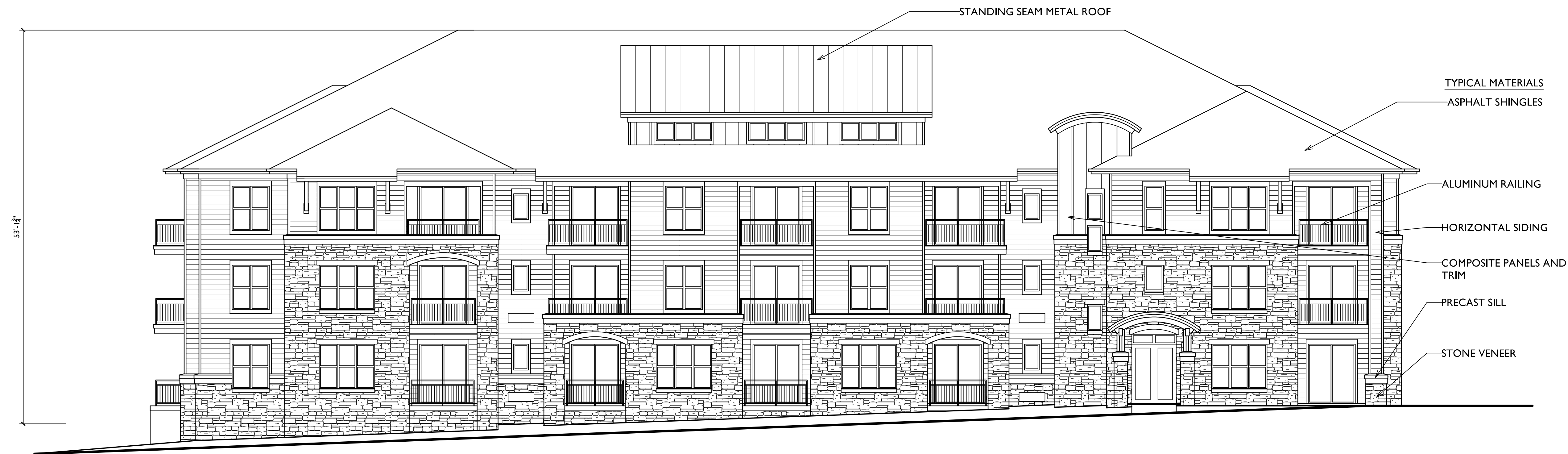
1 SOUTH ELEVATION - BUILDING 4 SCALE: 1/8"=1'-0"
