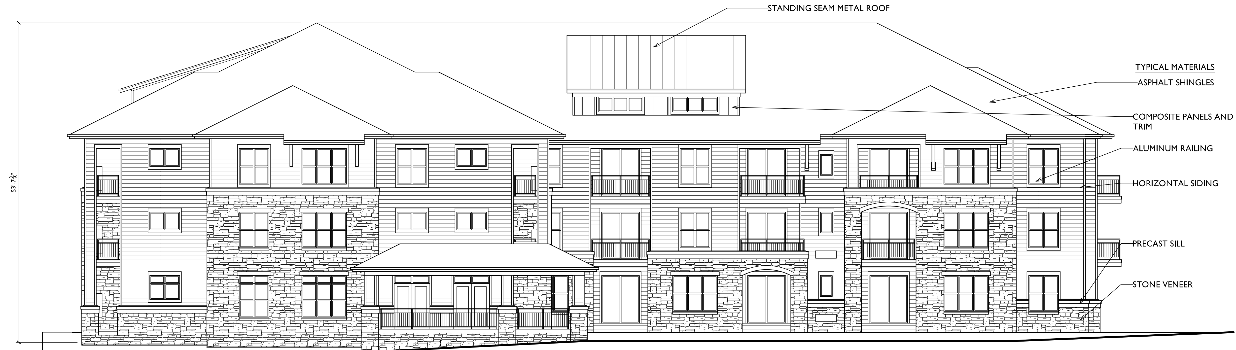
SOUTH ELEVATION - BUILDING 3 SCALE: 1/8"=1'-0"
