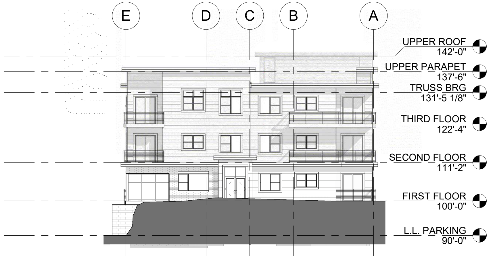
② EAST BUILDING ELEVATION-UDC 1/16" = 1'-0"
