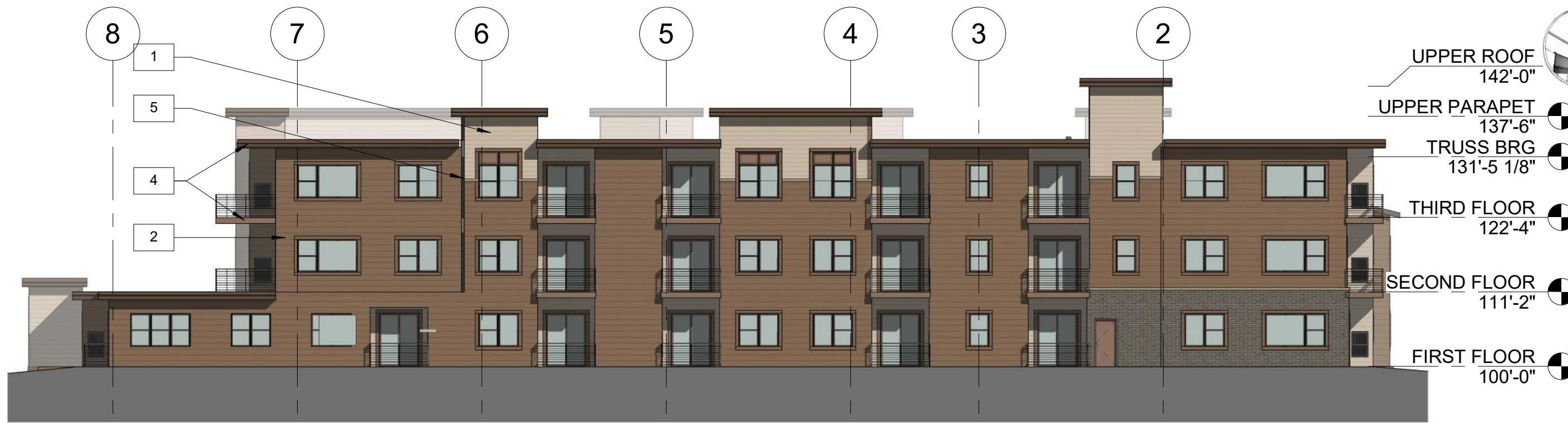
NORTH BUILDING ELEVATION-UDC COLOR 1/16" = 1'-0"
