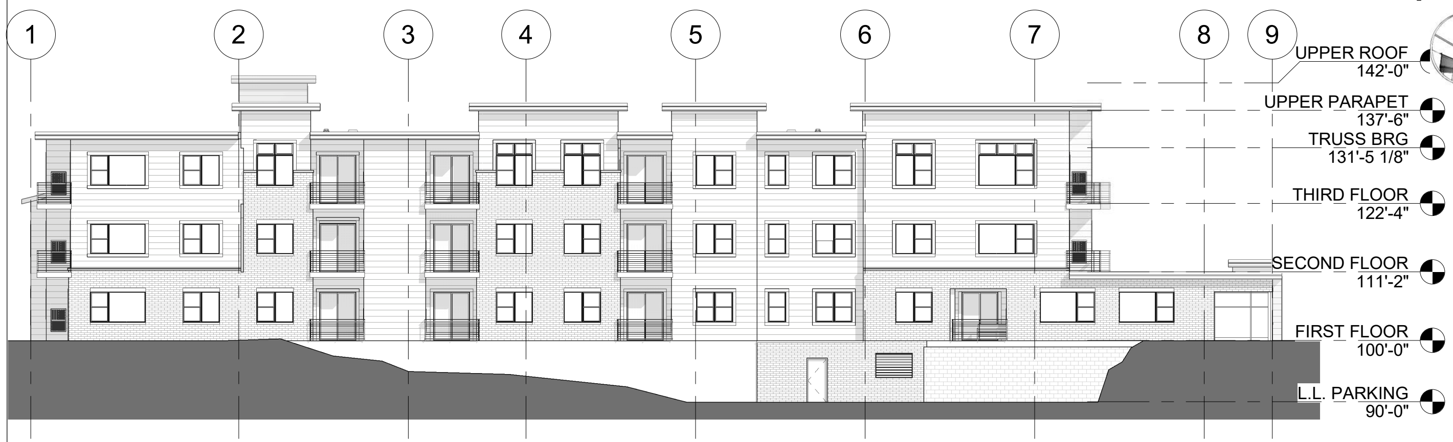
1 SOUTH BUILDING ELEVATION-UDC 1/16" = 1'-0"
