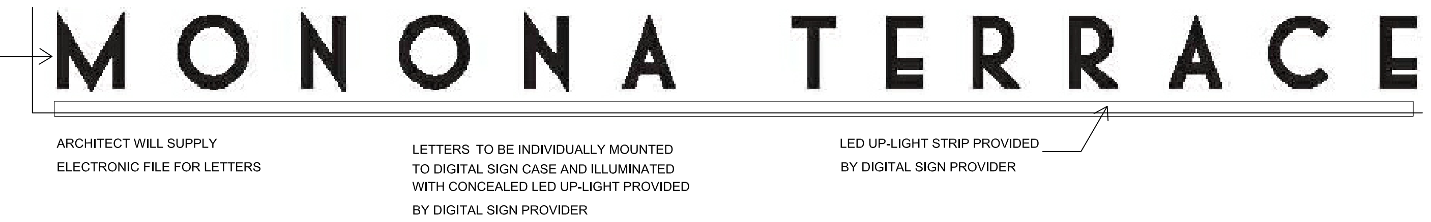
7 FREE STANDING LETTERING DETAIL Scale: 3/4"=0" (BY OTHERS)
