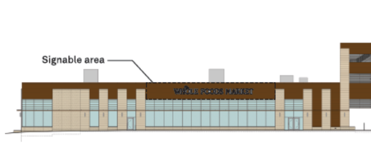
① SOUTH ELEVATION - COMPLIANT (120 SQ. FT.) SCALE: 1/32" = 1'-0"
