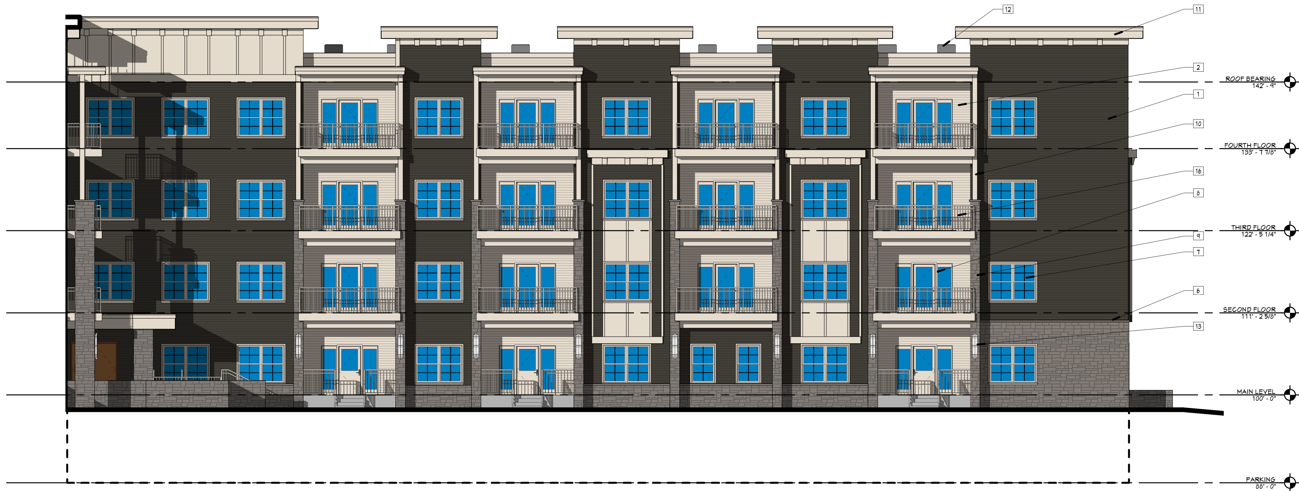
2 BUILDING 1 - EAST ELEVATION (BLDG 2 SIM) A4.2 1/8" = 1'-0"
