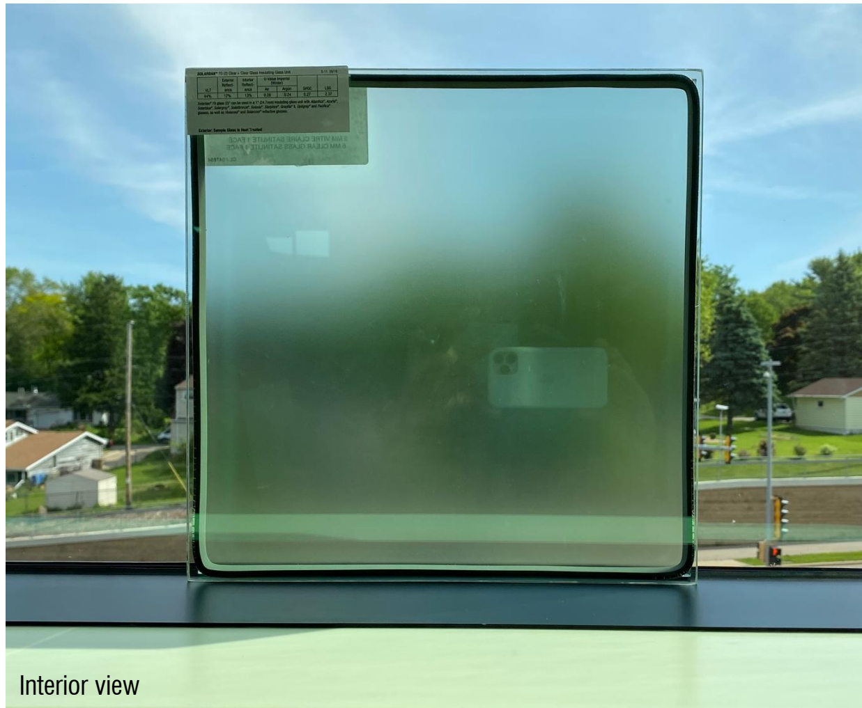
Translucent Glass: Solarban 70 with Satinlite-1 on 3 rd surface
