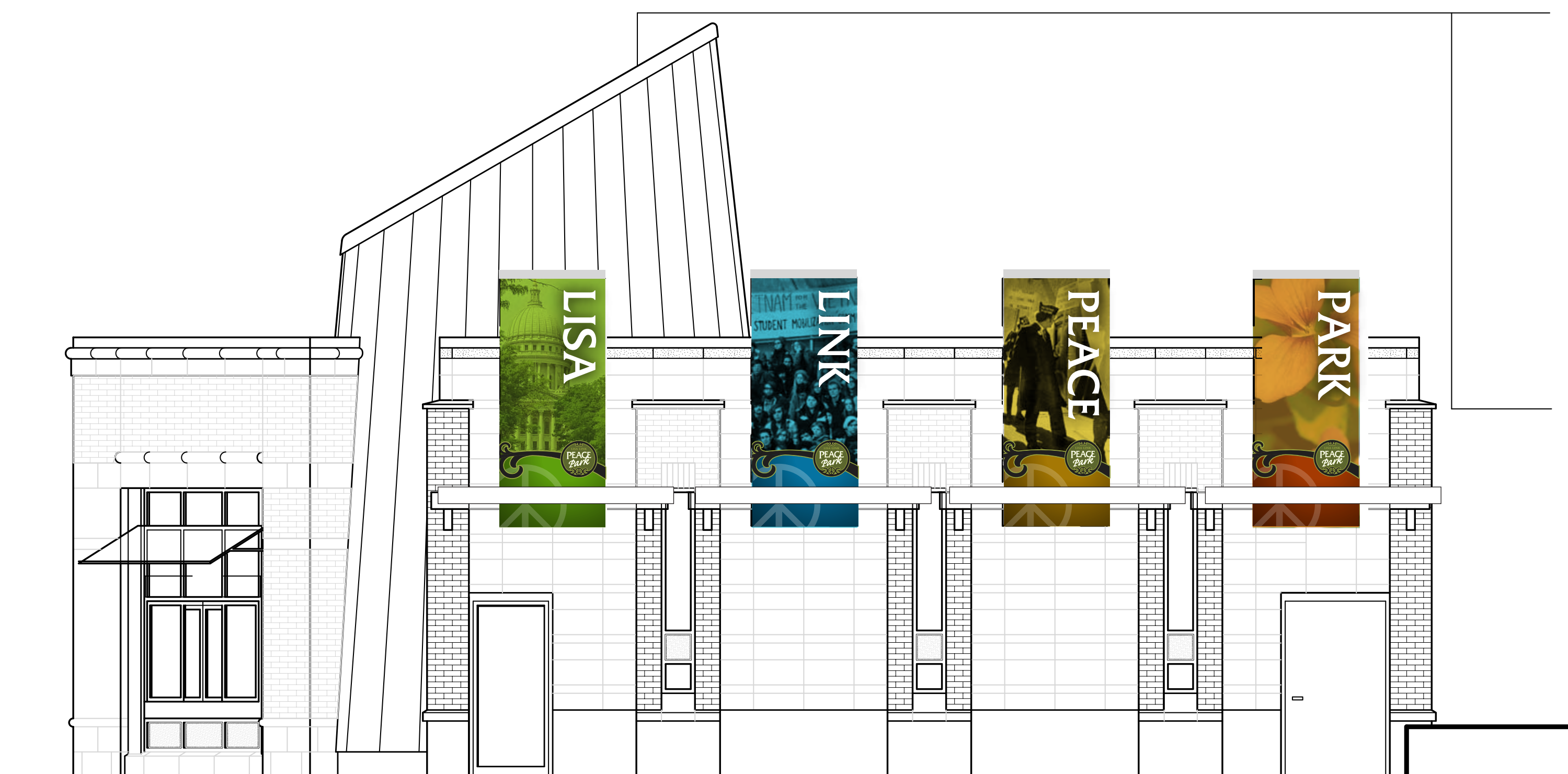
Exterior Banner Graphics: 4 quantity graphic banners facing the park Digital printed graphics to 10' tall x 4' wide aluminum panel (Dibond or vender recommended aluminum panel to withstand elements) Panels mount to building facade (masonry wall) and extend higher than the facade
