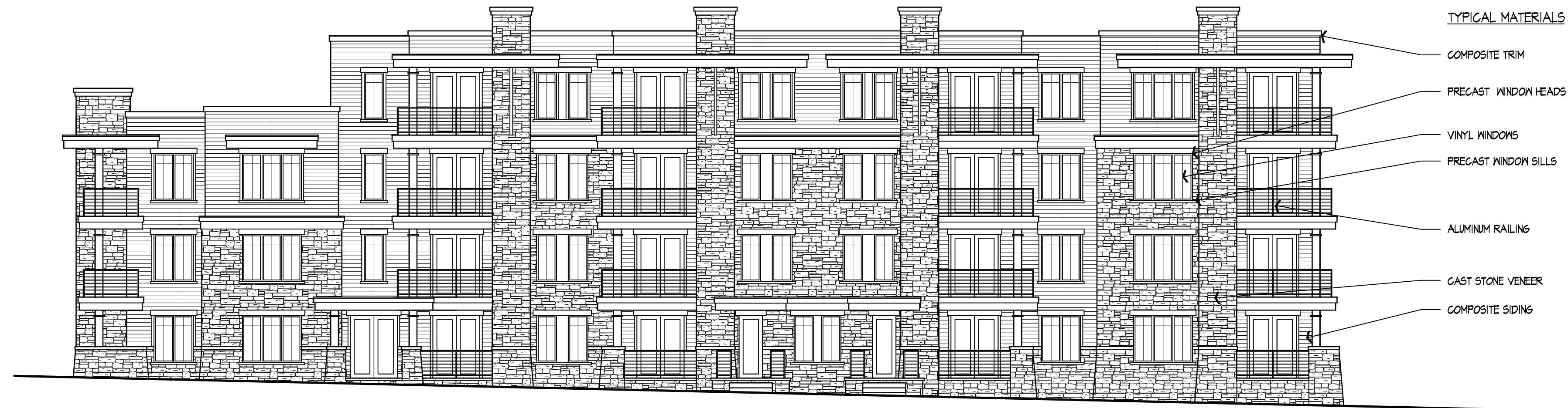
NORTH ELEVATION (ALONG MAYO DRIVE) 3/8" = 1'-0"
