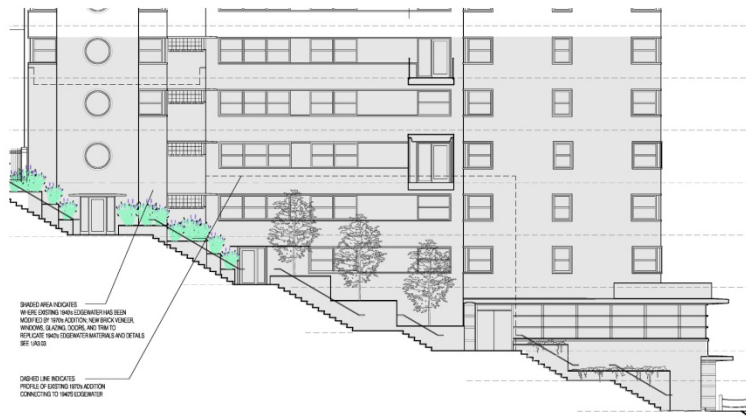
1 Partial Enlarged Elevation at New Construction SCALE: 1/8"=1'-0"
