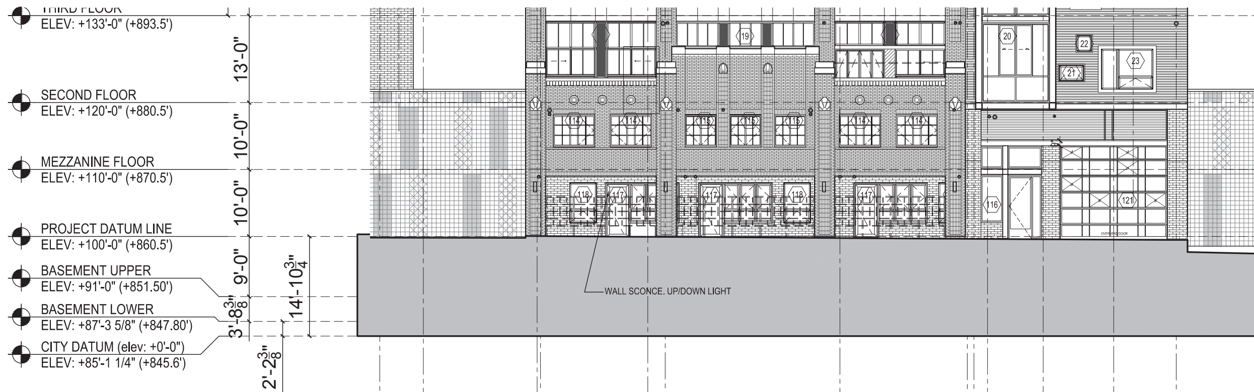
1 EXTERIOR ELEVATION (GILMAN STREET) STREET LEVEL SCALE: 3/32"=1'-0"
