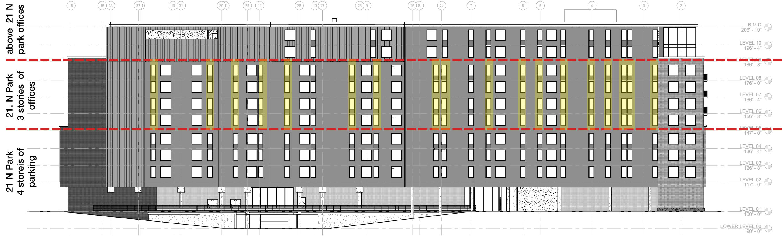
NORTH FACADE SHOWING ZONES OF NEIGHBORING OFFICE BUILDING
