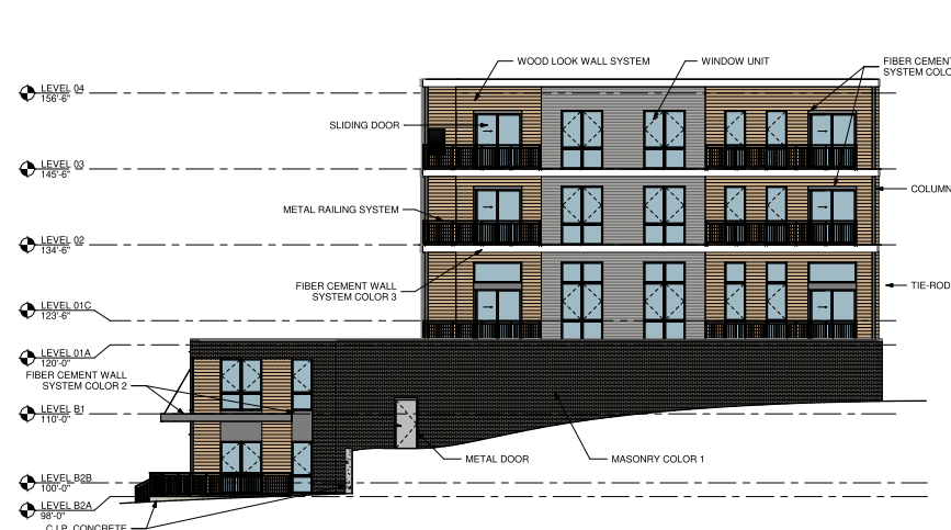
2 NORTH WING - WEST ELEVATION 1/8" = 1'-0"
