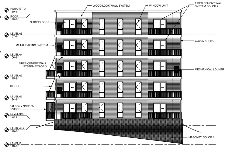
1 SOUTH WING - WEST ELEVATION B-W 1/8" = 1'-0"
