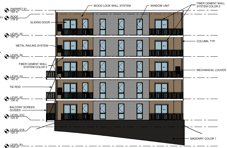
1 SOUTH WING - WEST ELEVATION 1/8" = 1'-0"
