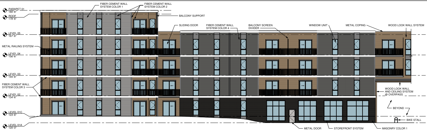
5 CENTRAL WING - EAST ELEVATION 02 1/8" = 1'-0"
