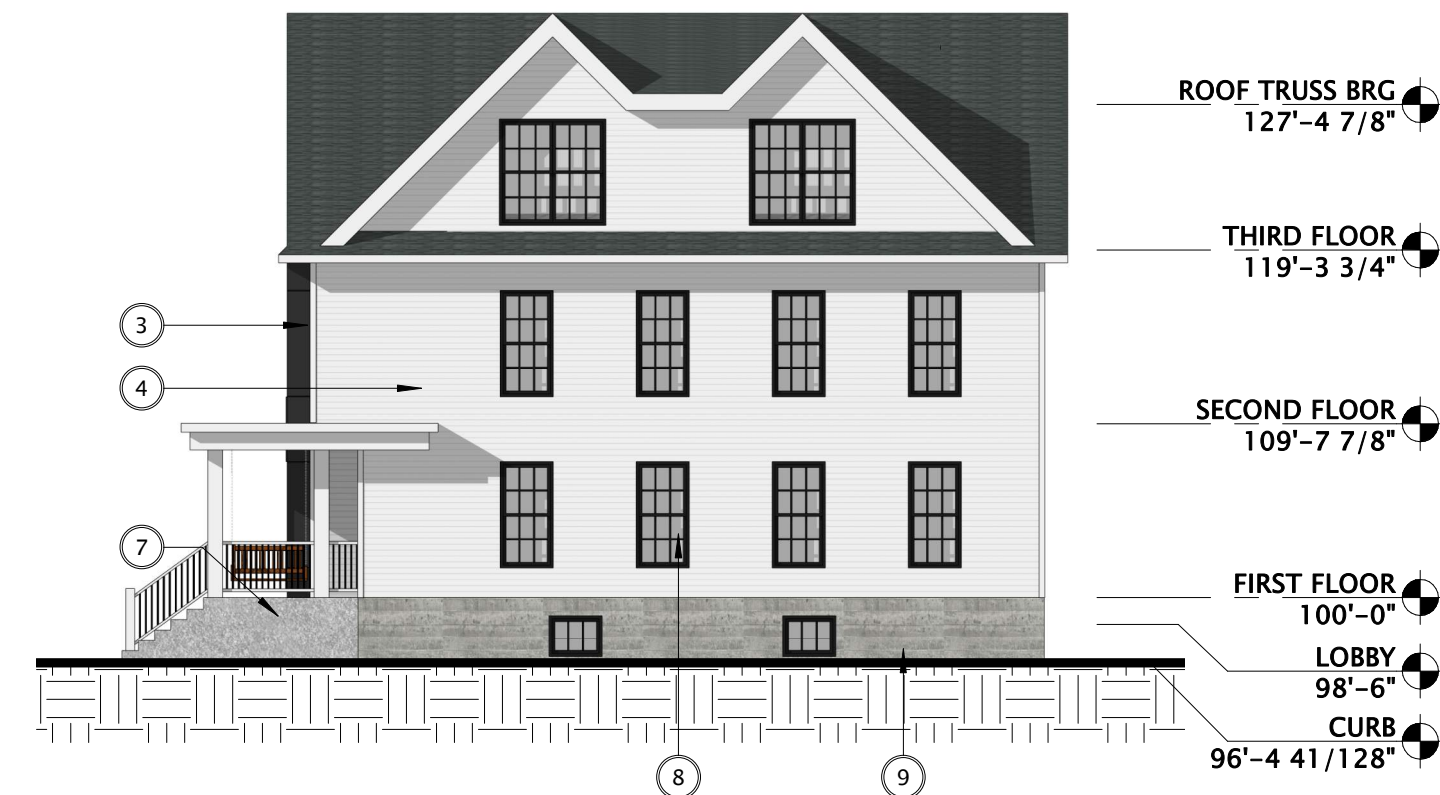
6 EAST ELEVATION NEW HOUSE - SKP 3/32" = 1'-0"
