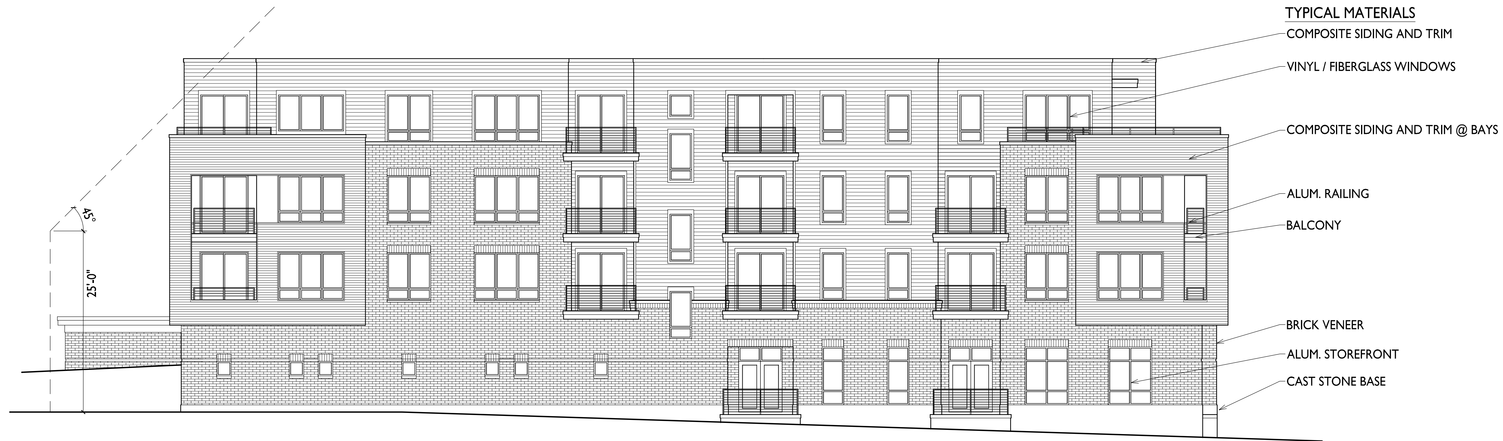
1 EAST ELEVATION A-2.3 1/8" = 1'-0"
