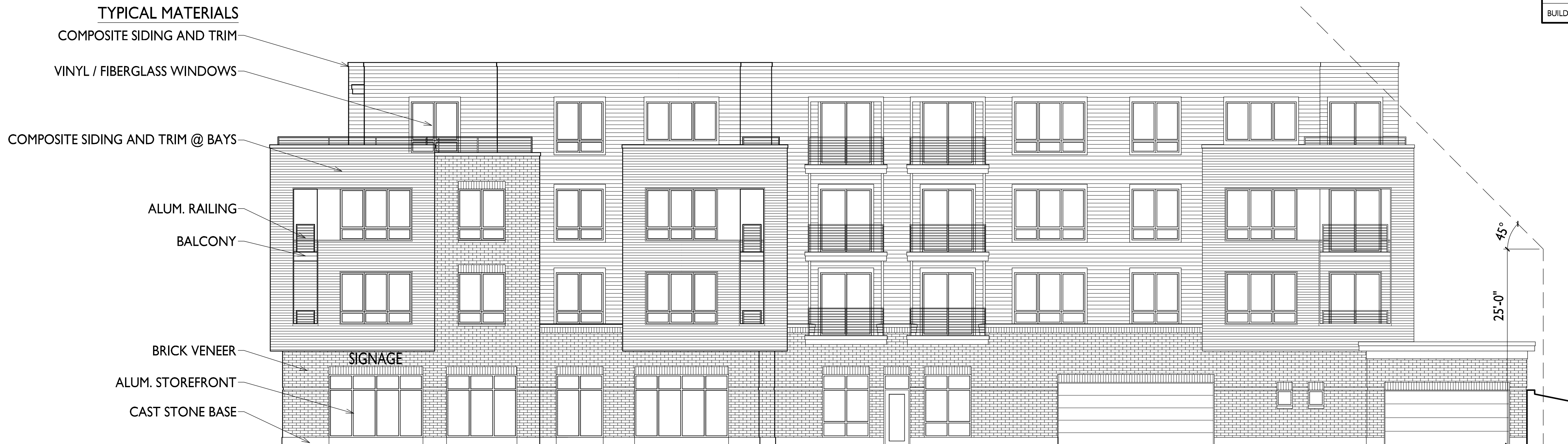
2 WEST ELEVATION ALONG CAPITAL DRIVE A-2.1 1/8" = 1'-0"
