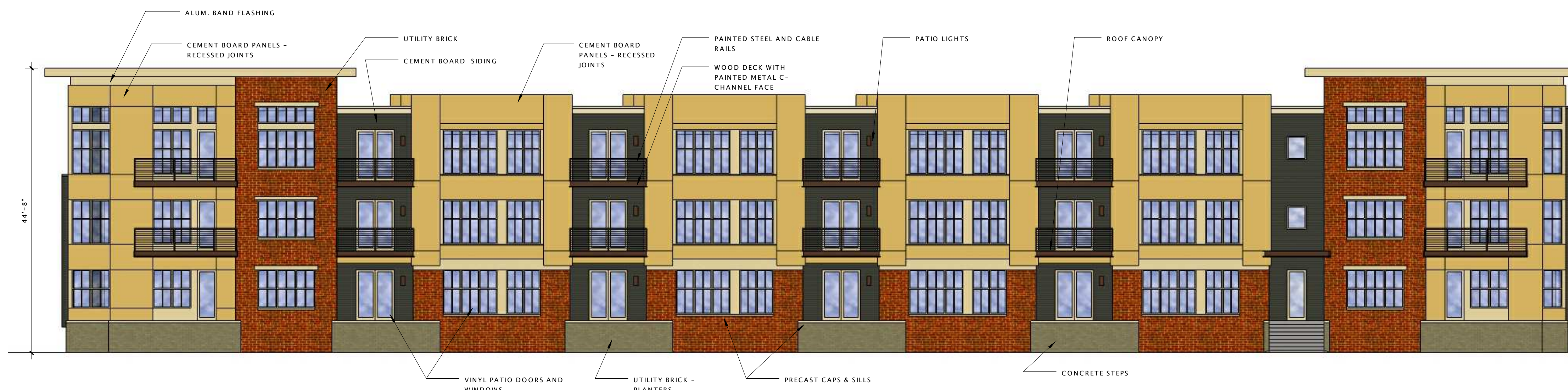
① Building B - Back Elevation 3/32" = 1'-0"
