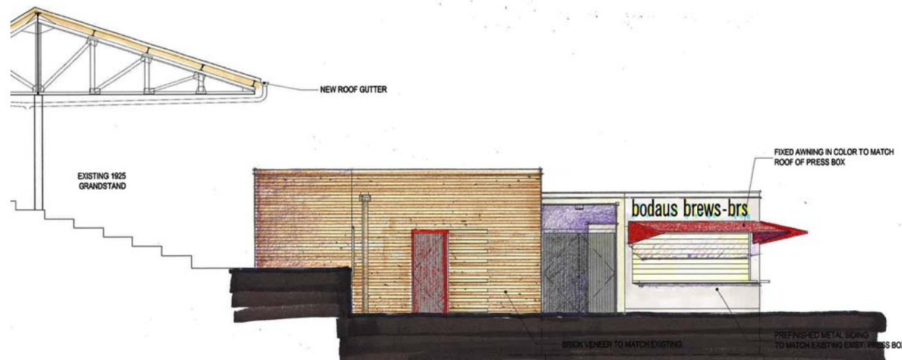
2 SOUTH ELEVATION - CONCESSIONS ADDITION Scale: 1/4"=1'-0"
