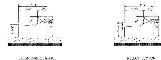
CONCRETE CURB & GUTTER NOT TO SCALE
