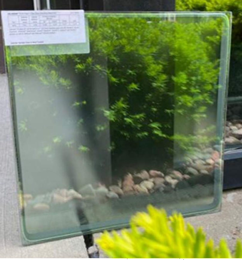
5 SOLARBAN 70 TRANSLUCENT GLASS SATINLITE 1 ON 3RD SURFACE (TO RECEIVE 2" X 4" BLACK BIRD GLAZING PATTERN)
