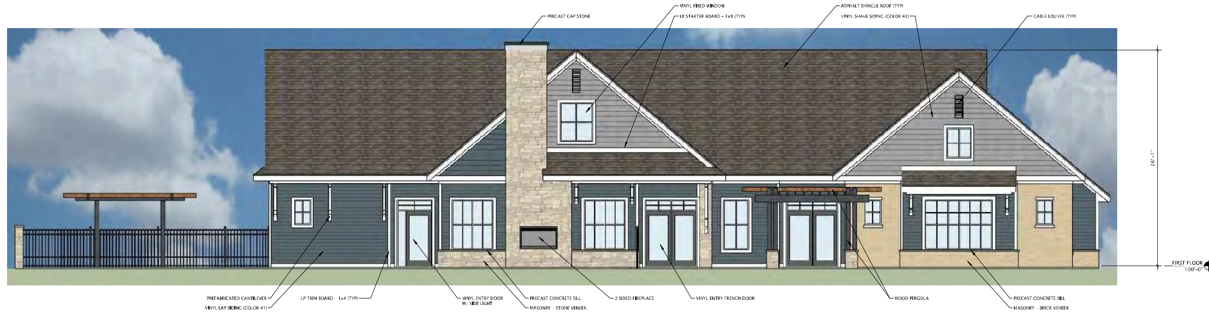
⑥ C - Elevation North 3/16" = 1'-0"
