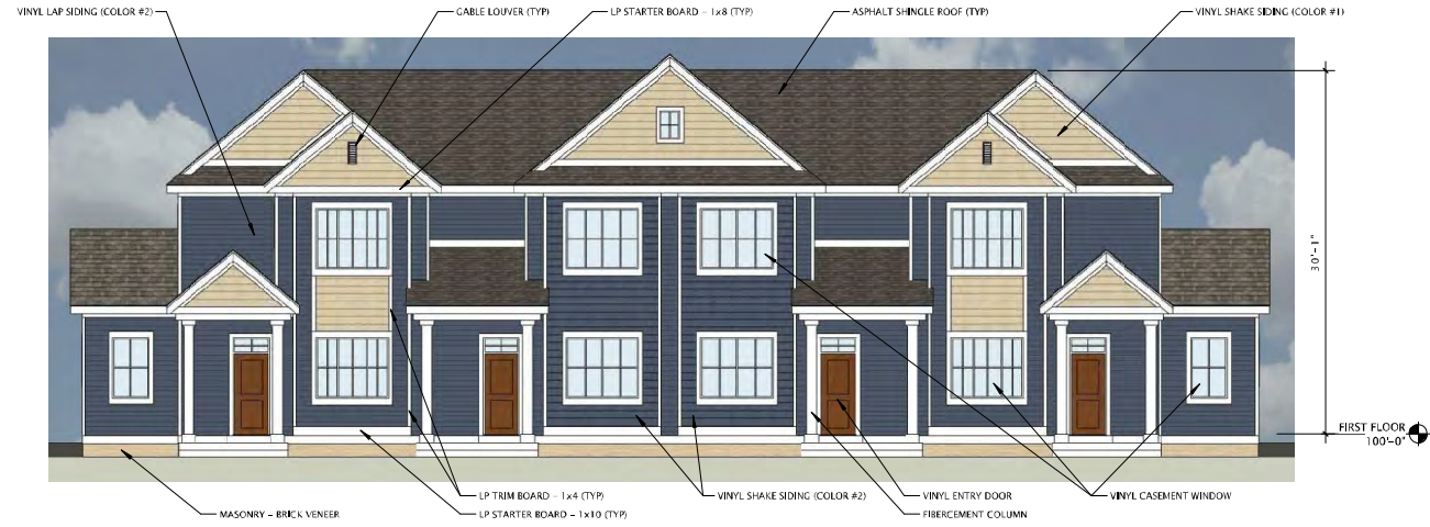
8 4 Unit West Elevation 1/8" = 1'-0"
