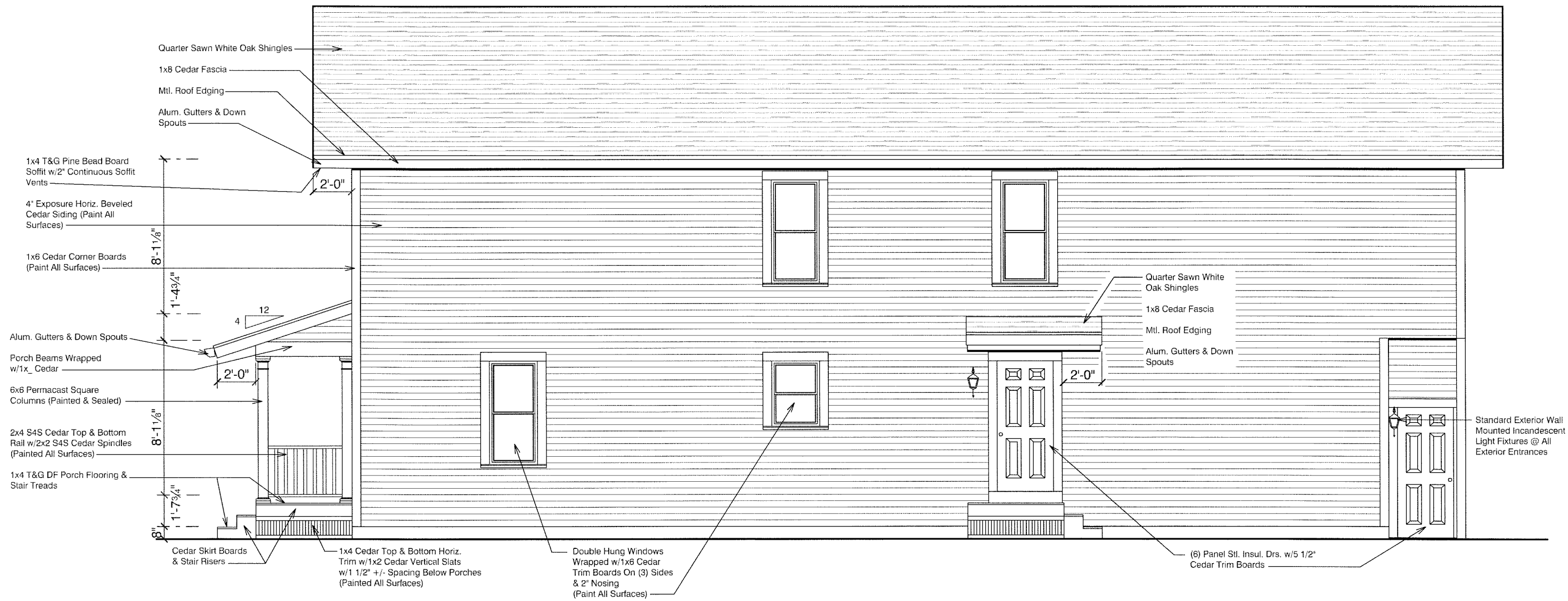
RIGHT ELEVATION Scale: 3/16" = 1'-0"
