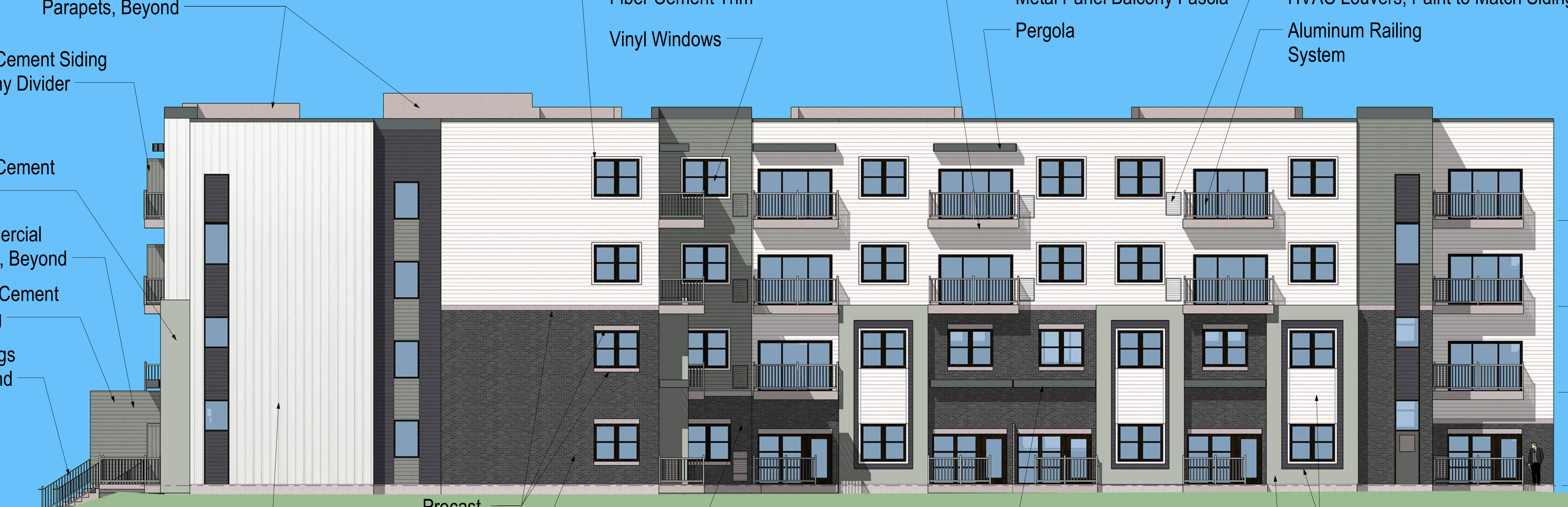
② Family Building - North Elevation 1/8" = 1'-0"
