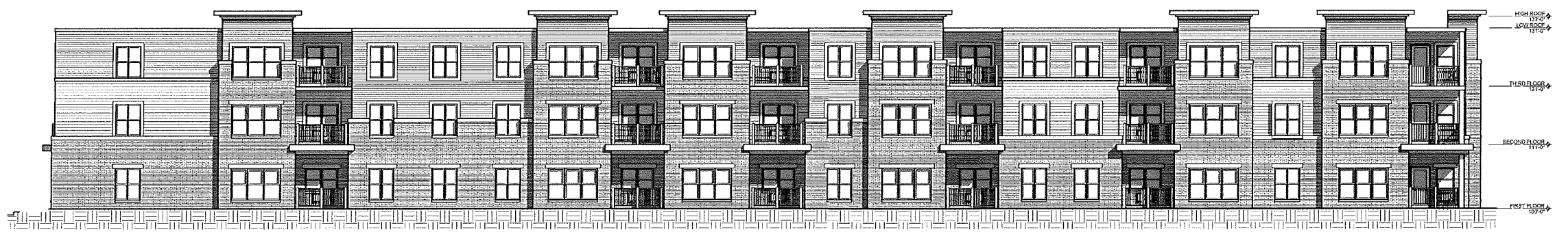
48 - UNIT SOUTH ELEVATION SCALE: 1/8" = 1'-0"
