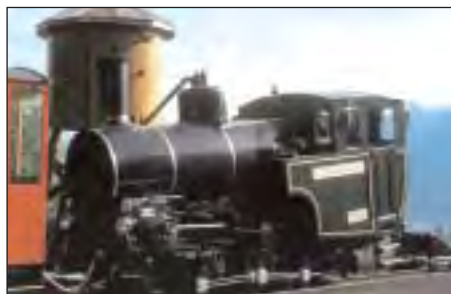
Fig. 13: Locomotive No. 1 of the Montreux – Glion – Rochers-de-Naye at Caux on its separate, non-electrified track. The rest of the line is electrified. Note the American style water tower with integrated fuel station.
