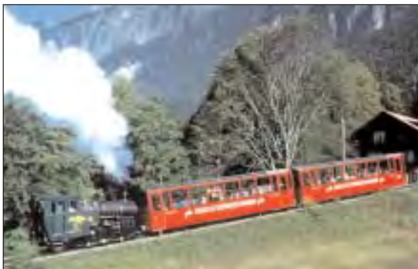
Fig. 12: Locomotive No. 12 of the Brien Rothorn with 120 passengers just outside Brien. White exhaust steam can be seen thanks to the cold outside temperature.
