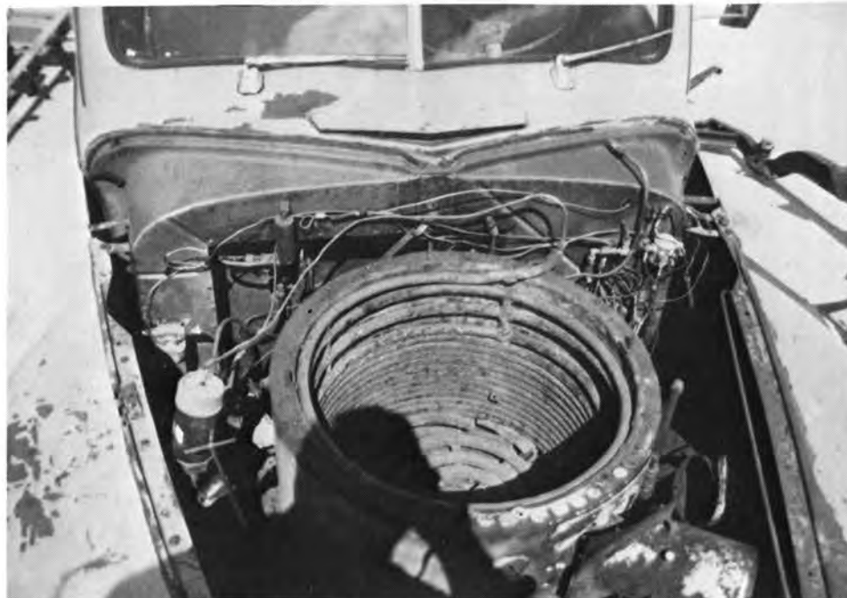
Steam generator (boiler) appears to have seen better days. Rust spots may indicate hood is missing entirely.
