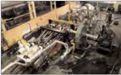
Fig. 26: Test stand with boiler, main steam pipe and steam engine exactly positioned as on the ship. The gear is from the obsolete diesel-electric drive and used here to increase the speed of the water brake.
