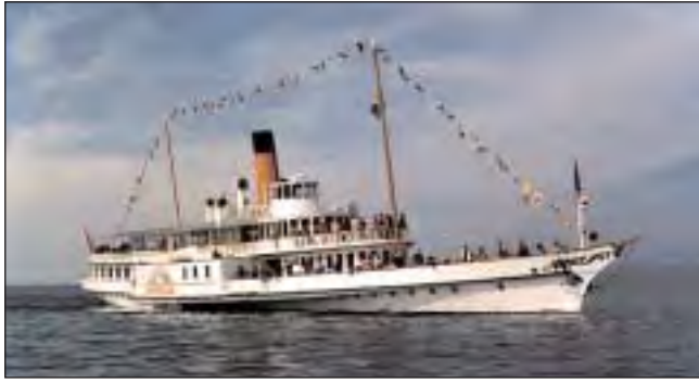
Fig. 25: Equipped with a new economic steam engine remote-controlled from the bridge, the entirely refurbished "Montreux" delights passengers, onlookers and accountants.
