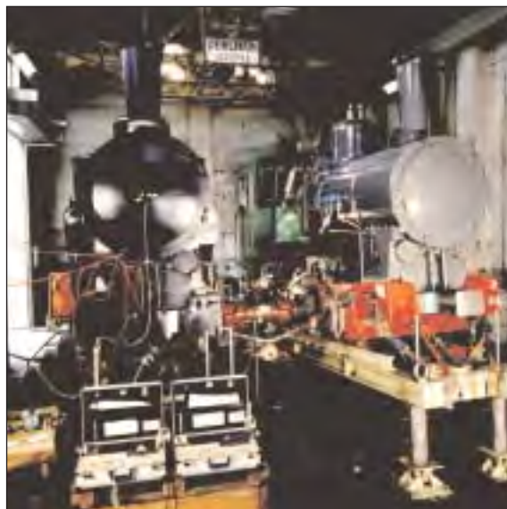
Fig. 10: Work load trials at SLM with locomotive No.12 of the Brienzt-Rothorn Railway on the left side and 999.201 of the Austrian Federal Railway. The two bright cases in the foreground contain the emission analysers.
