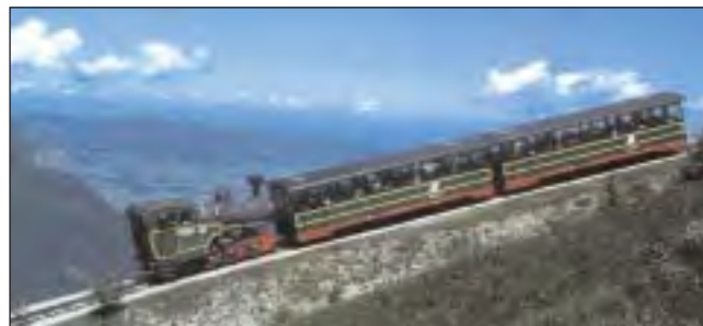
Fig. 14: Locomotive No. 999.201 of the Schafberg Railway with a full load of passengers on 1 in 4 grade. Note the clean combustion at full load.
