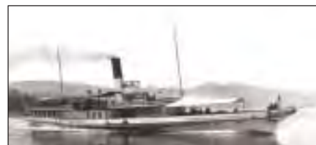
Fig.23: The "Montreux" was built in 1907 as a coal fired paddle steamer by the well-known Swiss company Sulzer Ltd.
