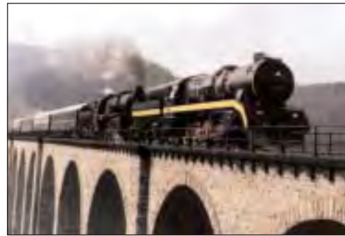
Fig. 22: Modernised oil-fired 52 8055 leads un-rebuilt coal-fired 52 7596 on the Orient Express. Each time a coal fired locomotive was used, the entire train had to be cleaned from soot and coal particles. Using 52 8055 saved a lot of man-hours of train cleaning alone.
