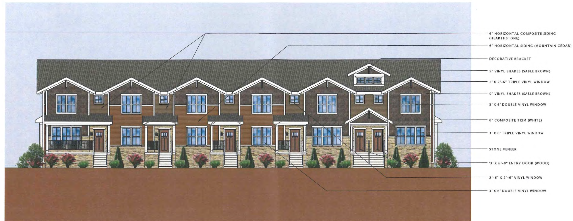
⑥ BUILDING 'E' - FRONT ELEVATION 1/8" = 1'-0"
