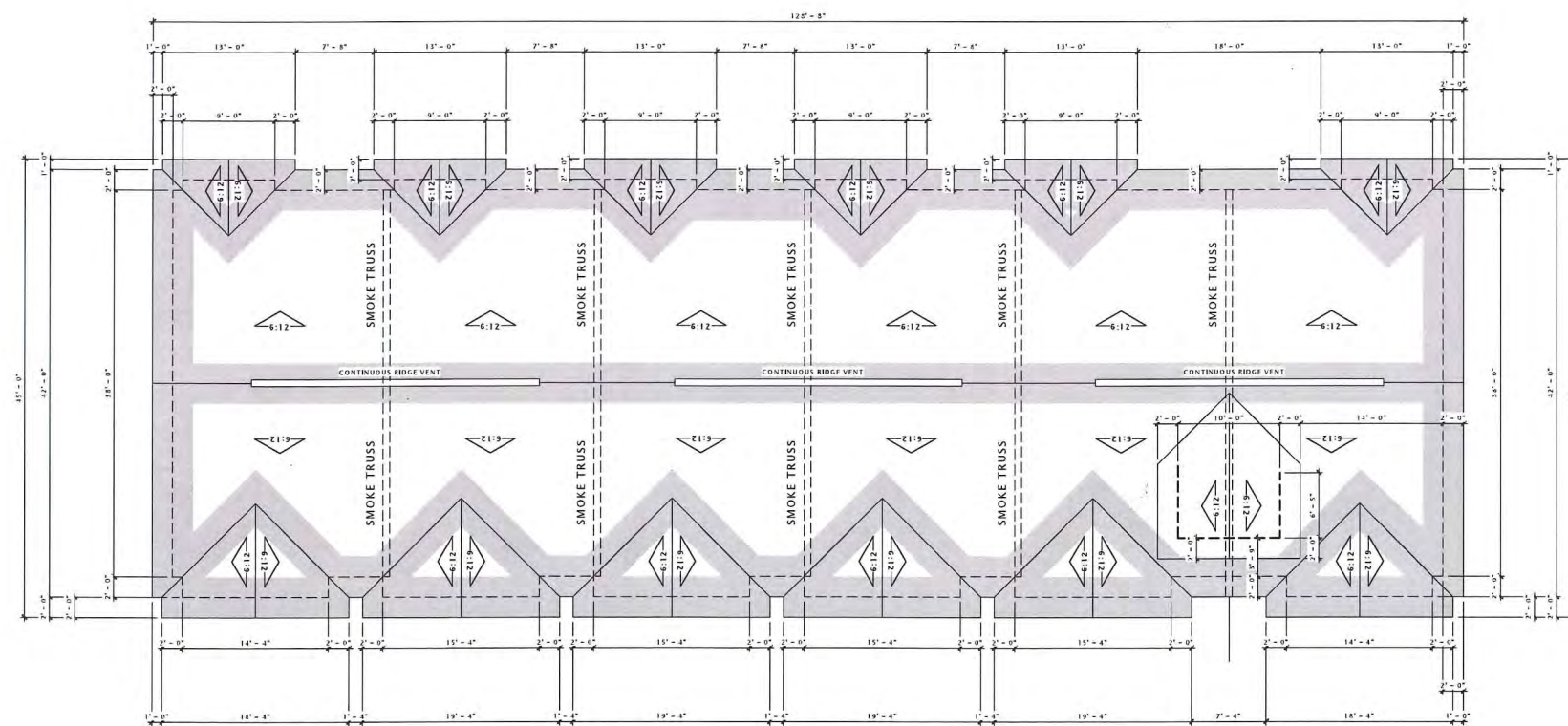
17 03 - ROOF PLAN - BUILDING 'E' 1/8" = 1'-0"
