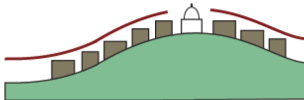
Skyline effect resulting from establishing maximum building heights relative to the natural topography of the Isthmus.
