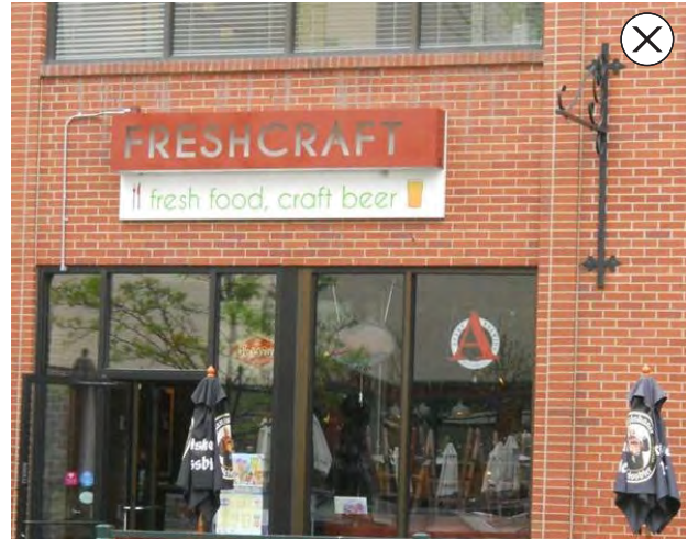
146. Remove remnants of old signage that will not be reused, such as the unused sign bracket in the upper right of this photo, and do not run exposed conduit on the exterior of the building.
