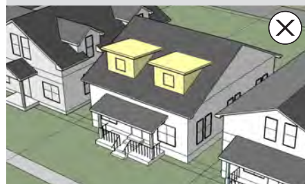
2. The new dormers illustrated above on the front-facing roof plane are inappropriate because they have shed roof style that is not seen in the surrounding historic context and visually overwhelm the original roof.
