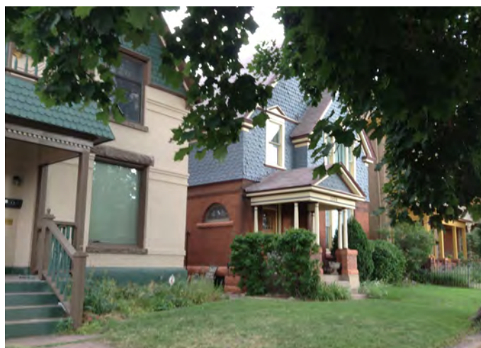
11. Glenarm Pl. streetscape. Note the uniformity in the front yard setback, the brick buildings with fish scale shingle in the upper stories, and projecting front porches of these Queen Anne style structures.
