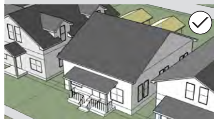
1. As illustrated above, new dormer(s) have been added to a rear-facing roof plane to be less visible from the street and sidewalk. A rear dormer or dormers may provide an opportunity for a small building addition as illustrated on page 66.
