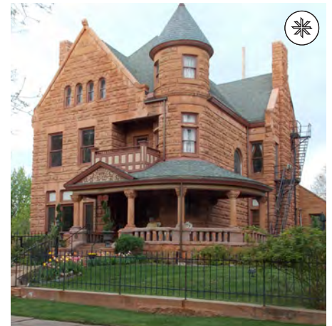
119. Locate and design a new retaining wall to minimize impacts on the historic context. As illustrated above, a low kick wall can help stabilize the yard while maintaining most of the historic slope.
