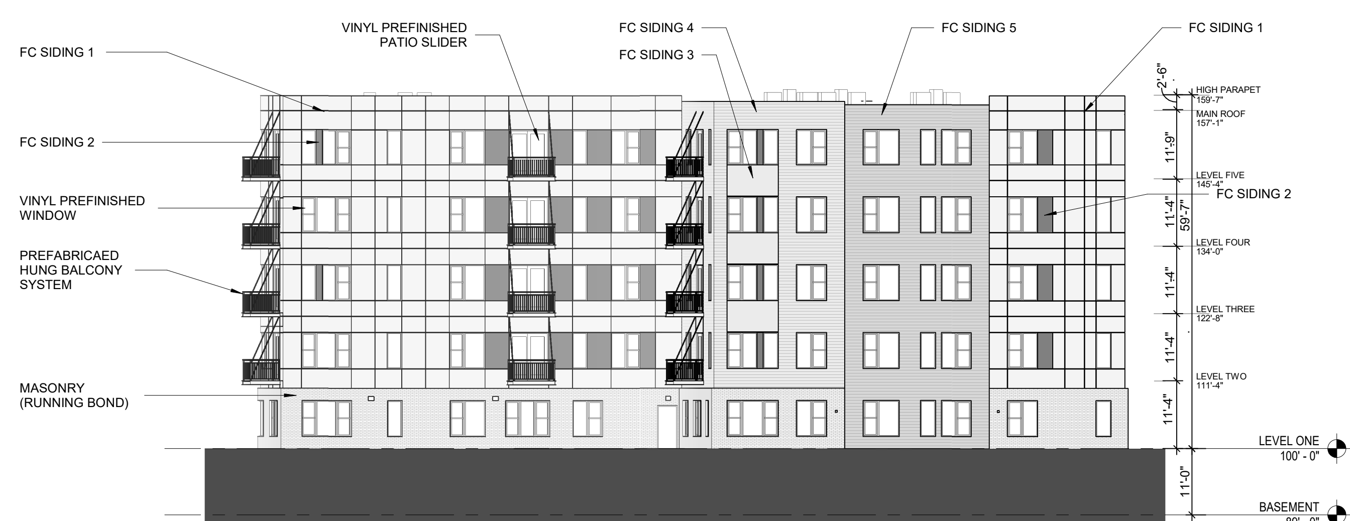
5 WEST ELEVATION - DESIGN SCALE: 1/16" = 1'-0"
