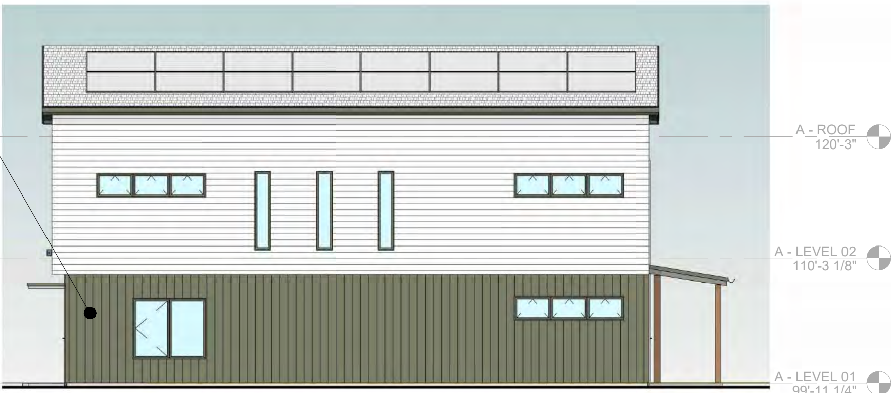
2D EXTERIOR ELEVATION - SOUTH 1/8" = 1'-0"
