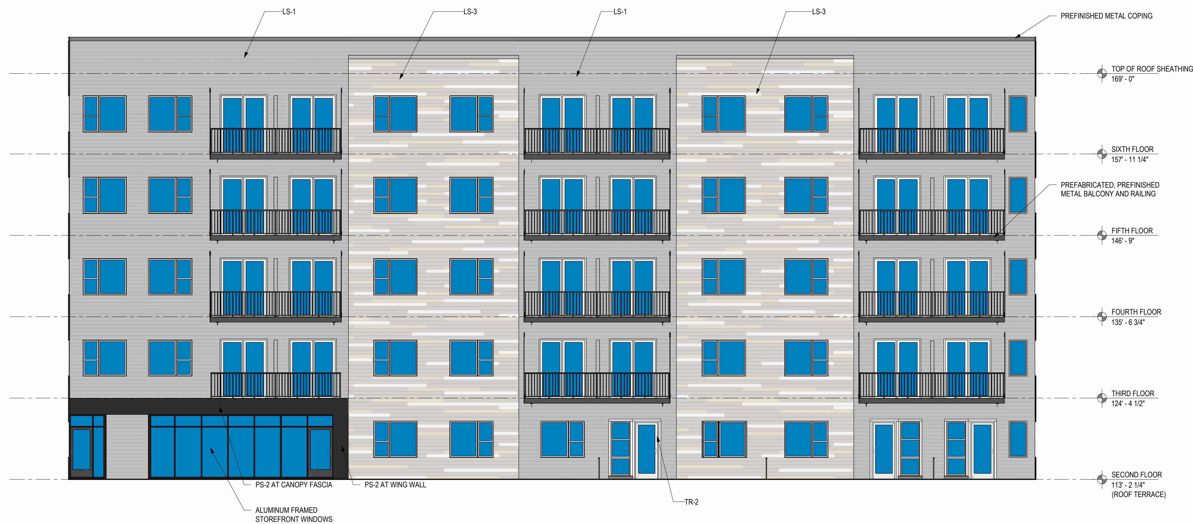
1 TERRACE SOUTH ELEVATION 1/8" = 1'-0"
