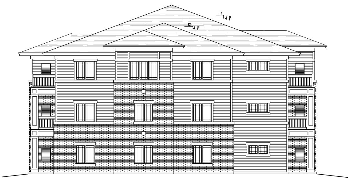
BUILDING A - WEST ELEVATION SCALE - 1/8" = 1'-0"
