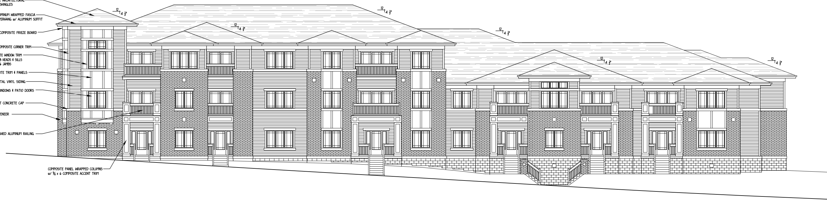
BUILDING A - NORTH ELEVATION (HERCULES TRAIL) SCALE - 1/8" = 1'-0"
