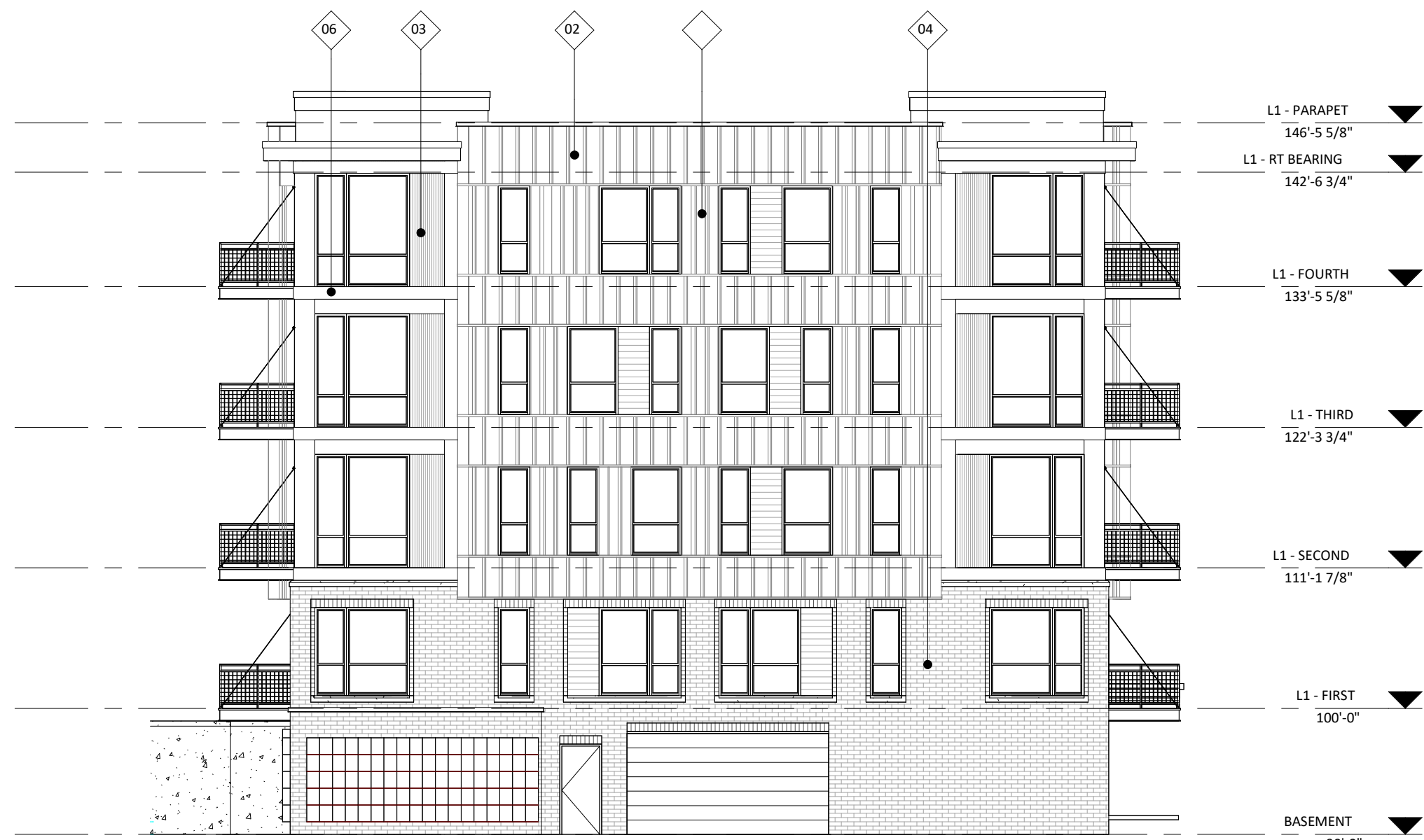
5 CITY ELEVATION - NORTHWEST AC202 3/32" = 1'-0"
