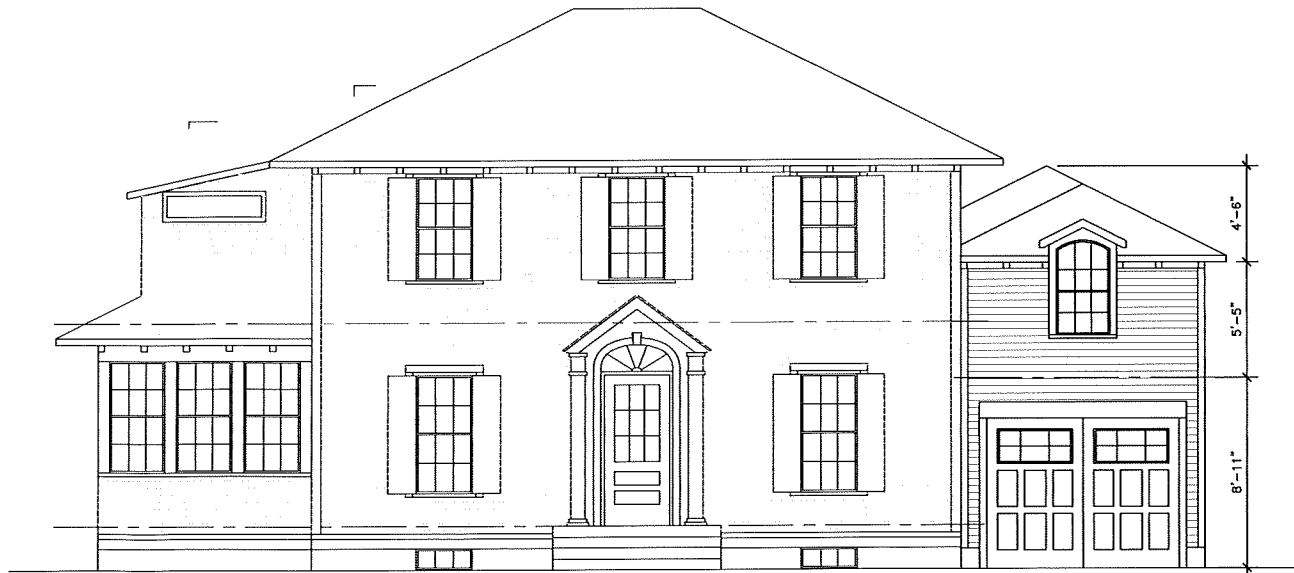
1 EAST EXTERIOR ELEVATION 1/4"=1'-0"
