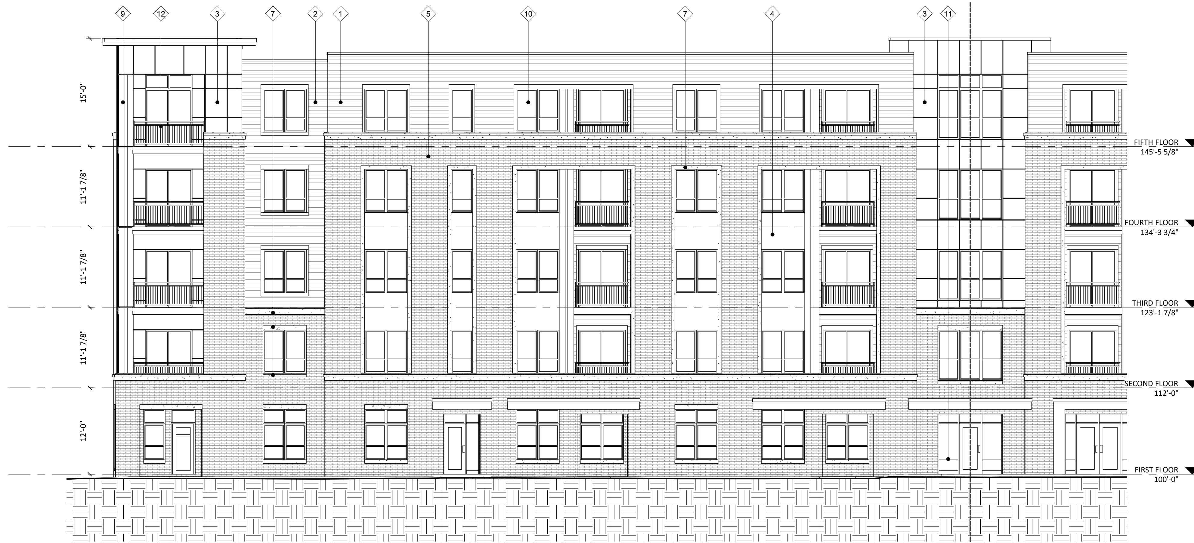
1 ELEVATION - NORTH WEST A201 1/8" = 1'-0"
