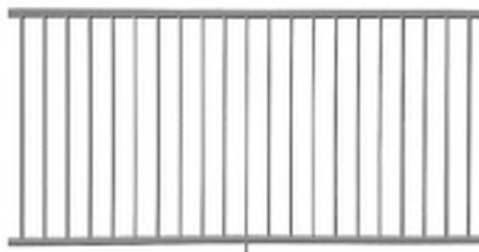
BLACK METAL GUARDRAIL (AT BALCONIES)
