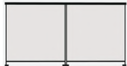
CLEAR GLASS GUARDRAIL (AT ROOFTOP AMENITY DECK)
