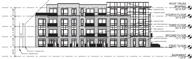
3 BUILDING #2 - EAST ELEVATION 1/16" = 1'-0"
