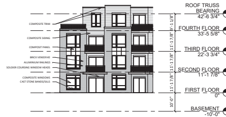
4 BUILDING #2 - EAST ELEVATION INTERIOR 1/16" = 1'-0"
