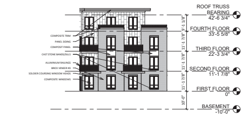
5 BUILDING #1 - WEST ELEVATION INTERIOR 1/16" = 1'-0"
