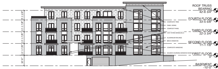
3 BUILDING #1 - EAST ELEVATION 1/16" = 1'-0"
