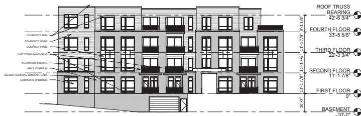
5 BUILDING #2 - WEST ELEVATION 1/16" = 1'-0"
