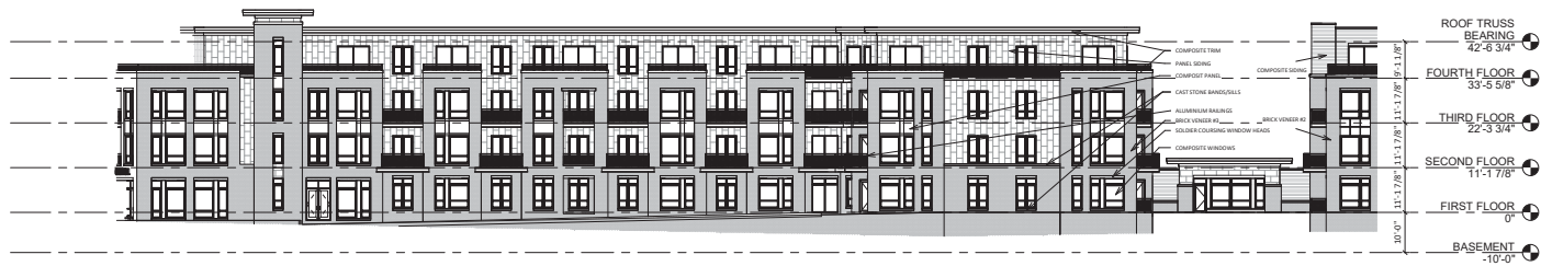
2 BUILDING #1 - SOUTH ELEVATION 1/16" = 1'-0"
