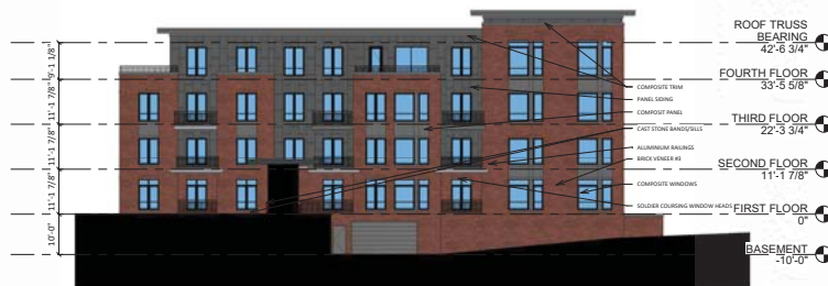
3 COLORED - BUILDING #1 - EAST ELEVATION A2.3 1/16" = 1'-0"
