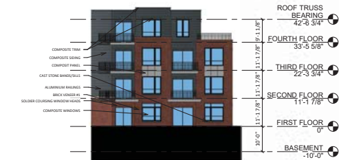
6 A-2.4 COLORED - BUILDING #2 - WEST ELEVATION INTERIOR 1/16" = 1'-0"
