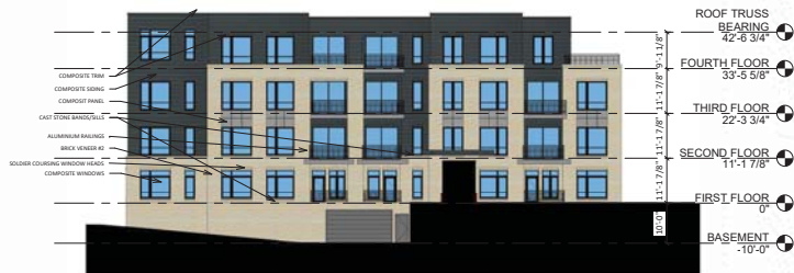
5 A-2.4 COLORED - BUILDING #2 - WEST ELEVATION 1/16" = 1'-0"
