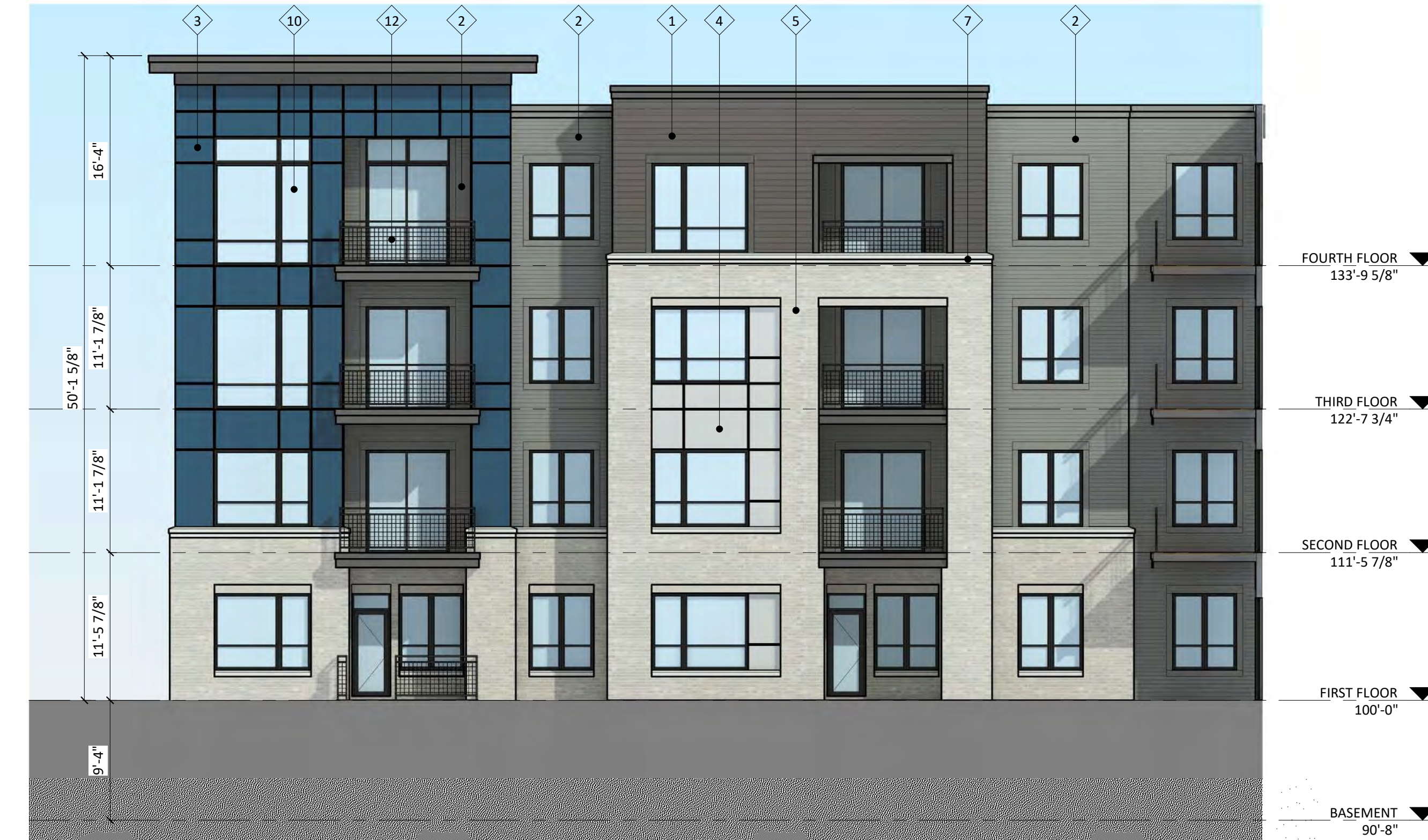
2 COLORED ELEVATION - TERRACE - SOUTH A-2.7 1/8" = 1'-0"
