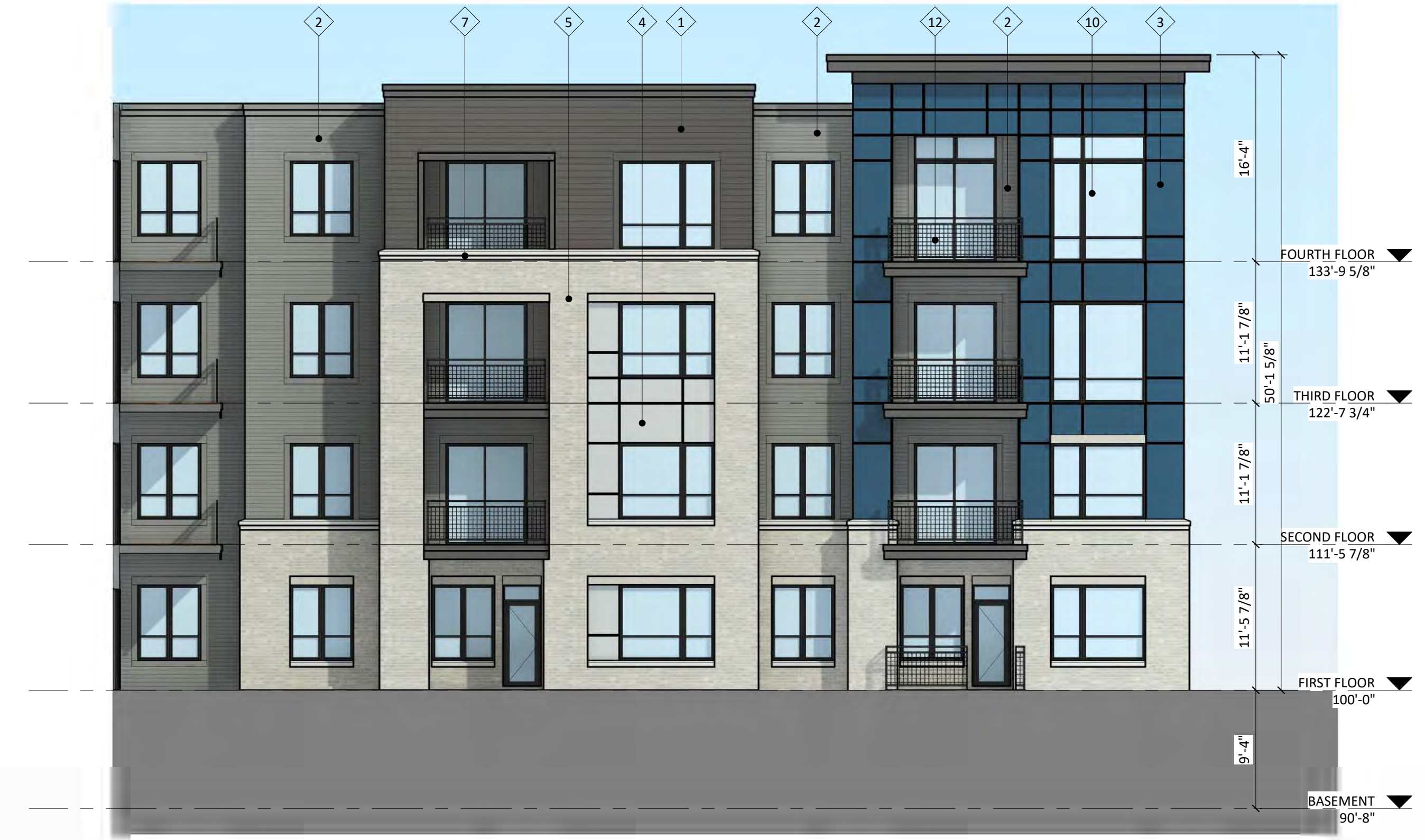
2 COLORED ELEVATION - TERRACE - NORTH A-2.8 1/8" = 1'-0"
