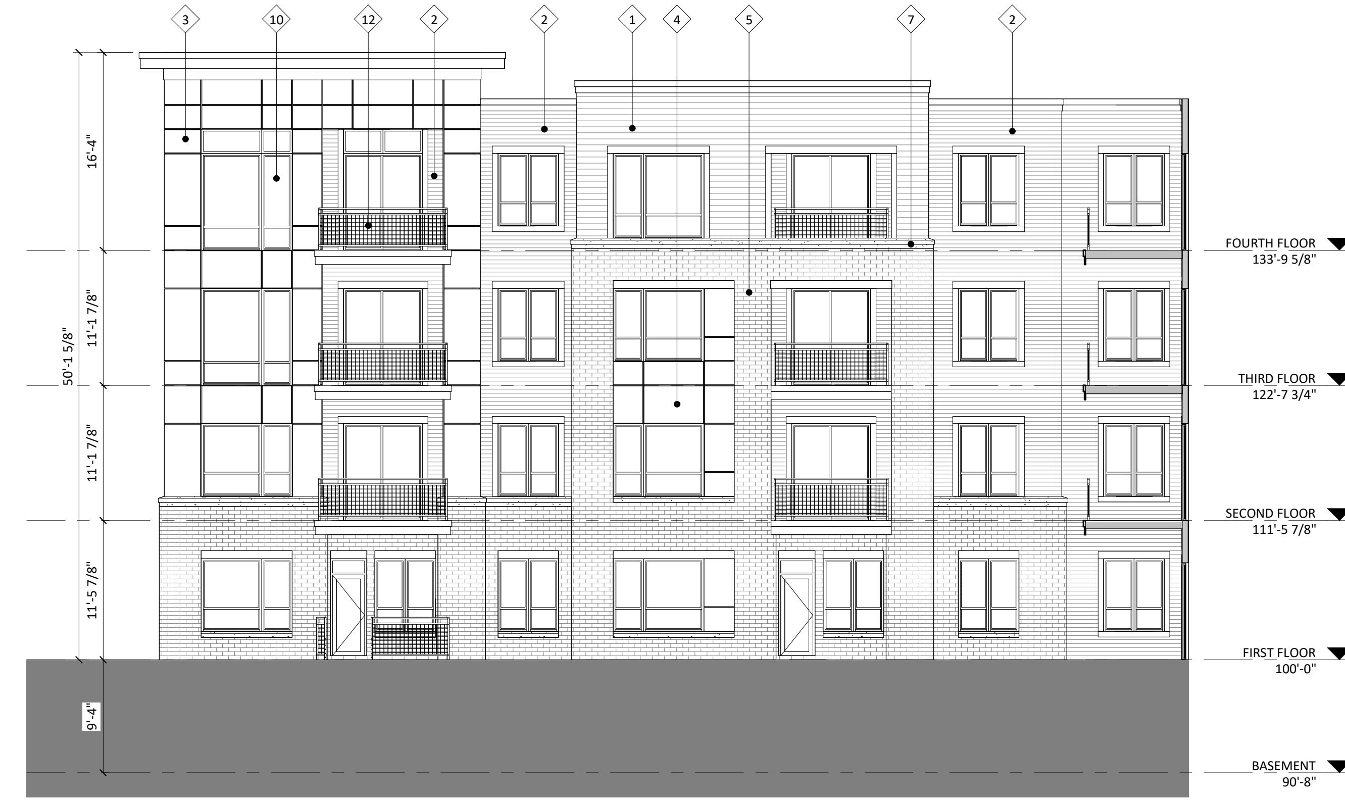
2 ELEVATION - TERRACE - SOUTH A-2.3 1/8" = 1'-0"
