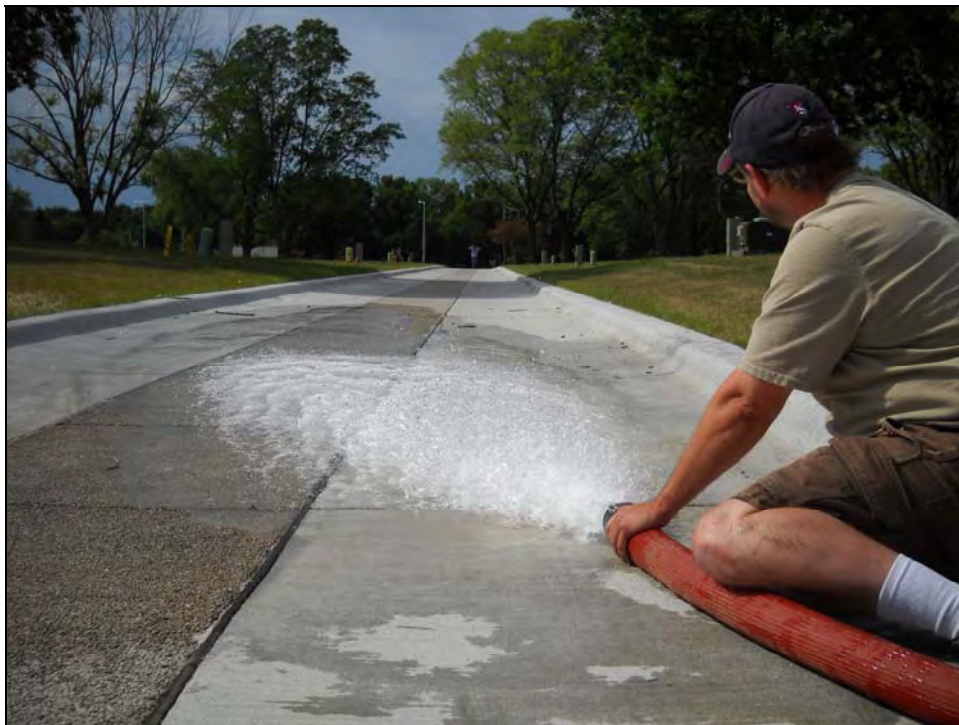
Photo 3: The end of wet pavement is visible, indicating all water has infiltrated.
