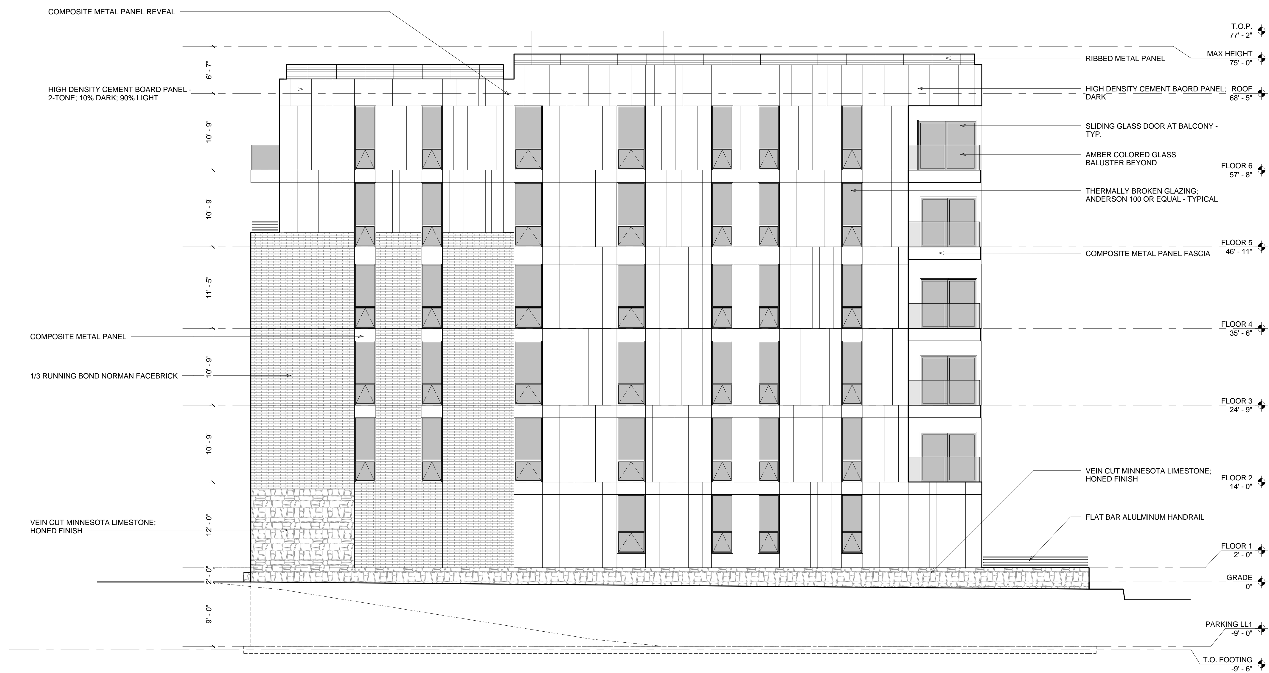
1 EXTERIOR ELEVATION - NORTH 1/8" = 1'-0"
