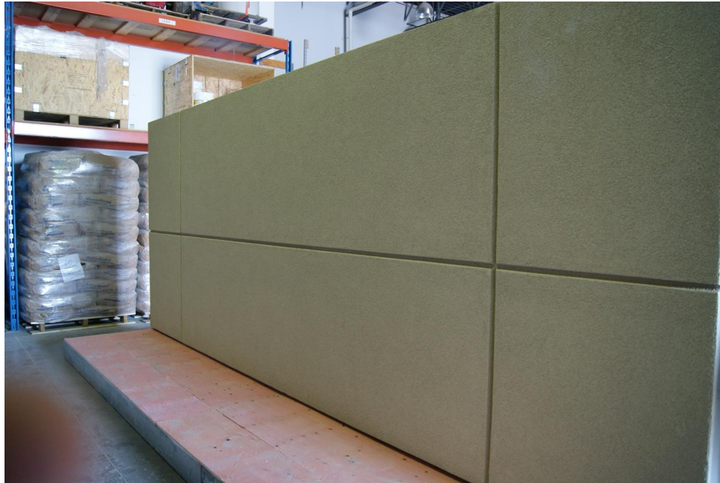
Mock-Up of E.I.F.S. -textured paint on left and flat finish on right
