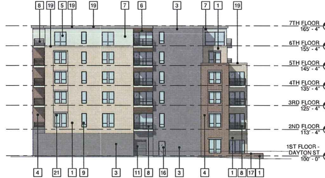
2 WEST ELEVATION - DAYTON BUILDING A202 1/16" = 1'-0"
