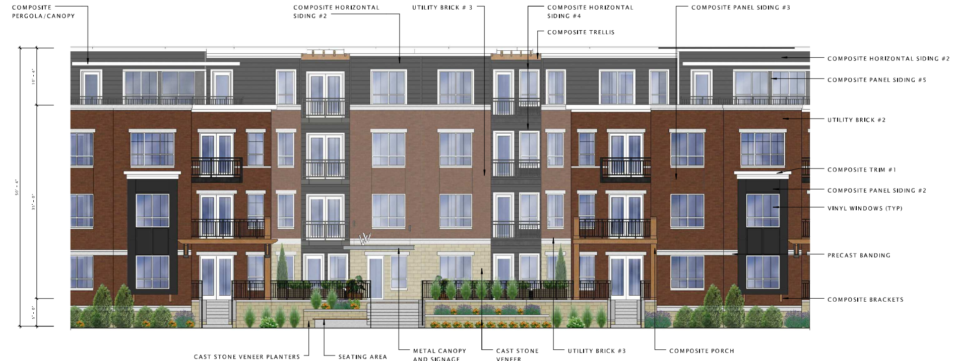
② Dayton Street Entry Enlarged Elevation 1/8" = 1'-0"
