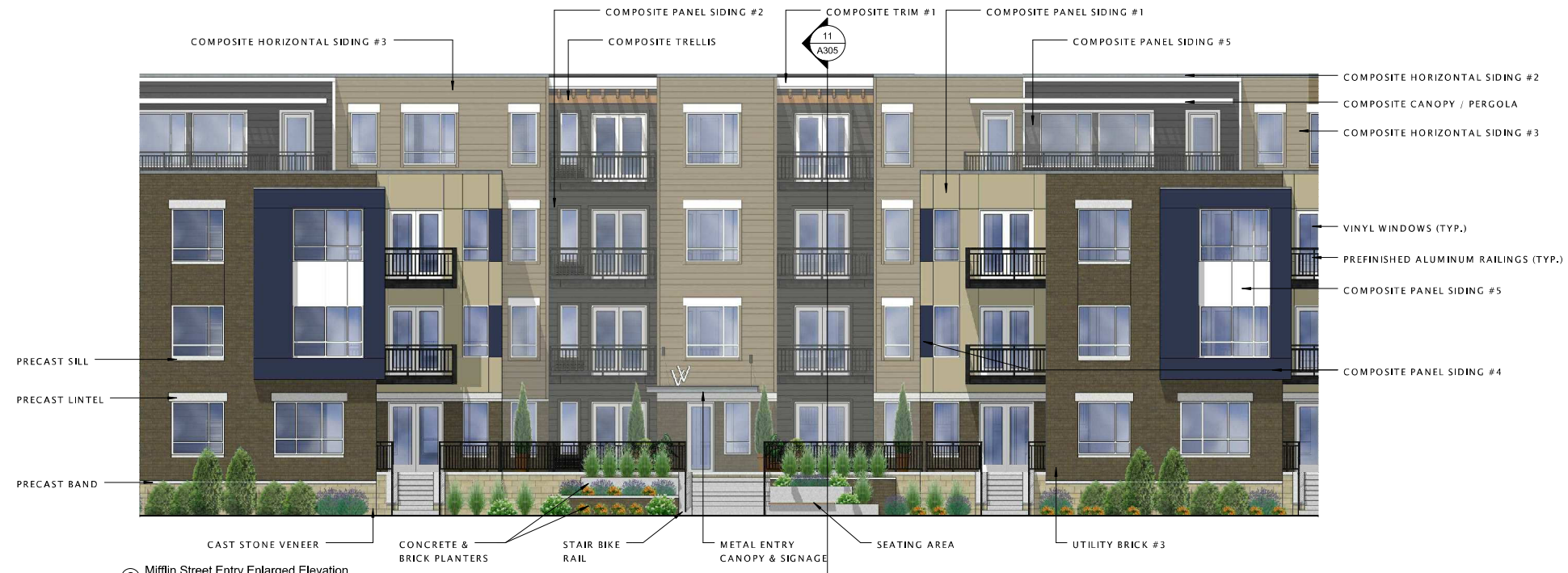
② Miffin Street Entry Enlarged Elevation 1/8" = 1'-0"
