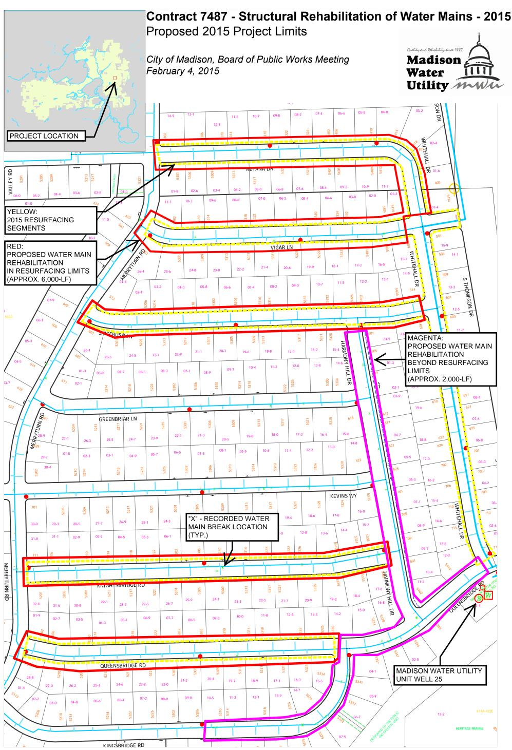
Madison Water Utility will be rehabilitating approximately 8,000-FT of existing, deteriorated water mains in the Unit Well 25 area using structural cured-in-place-pipe lining methods designed for pressurized drinking water applications. Approximately 6,000-FT of the project is located within 2015 street resurfacing segments and will be completed ahead of the proposed resurfacing. Estimated project cost: \$1,000,000.
