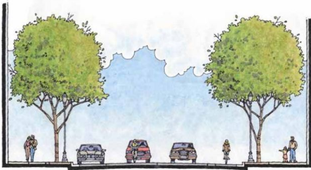
Figure 16. Wilson Street Cross Section with Parking on Street's North Side, Westbound Sharrow, and Eastbound Cycle Track
