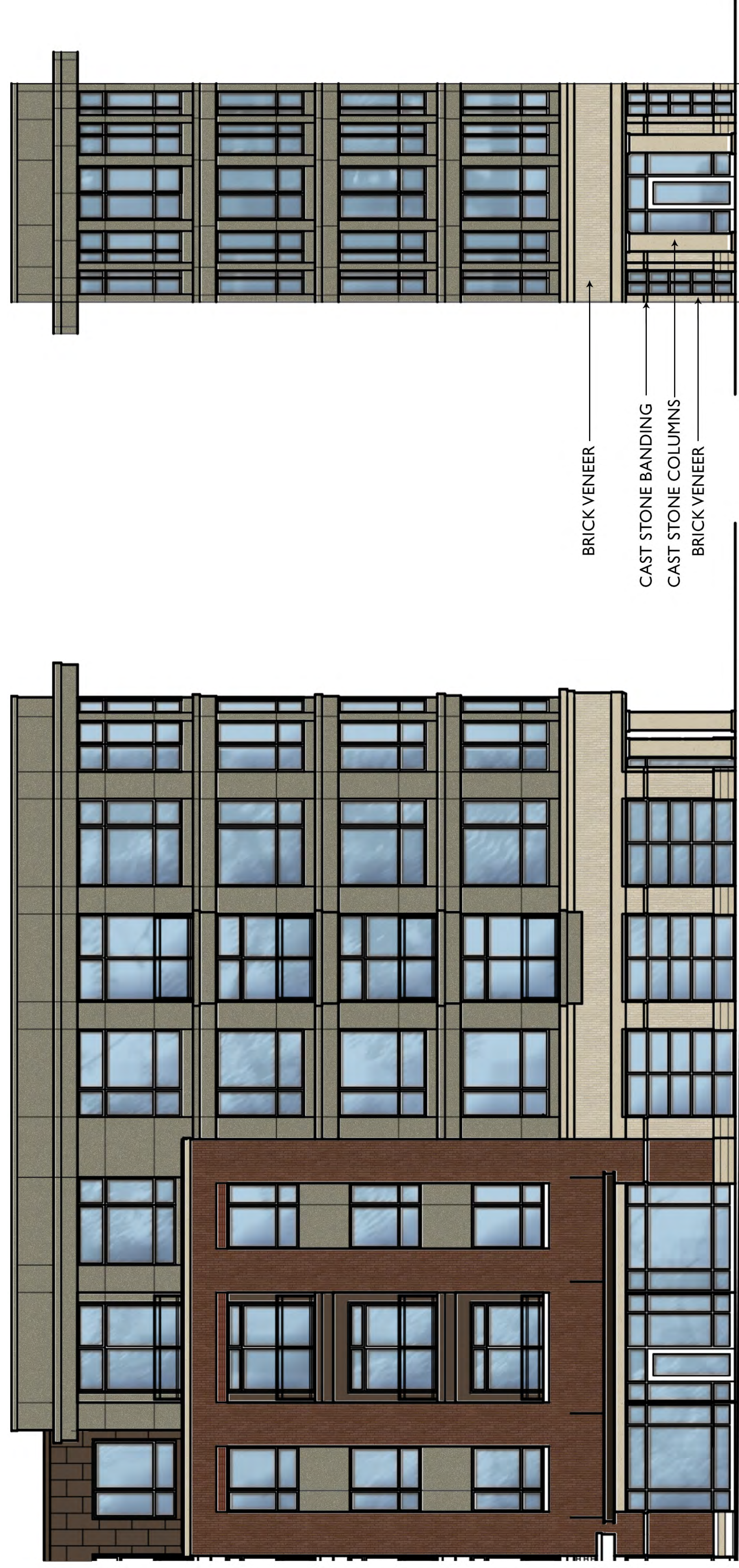
CORNER DETAIL - OPTION 2 - BRICK & CAST STONE BASE
