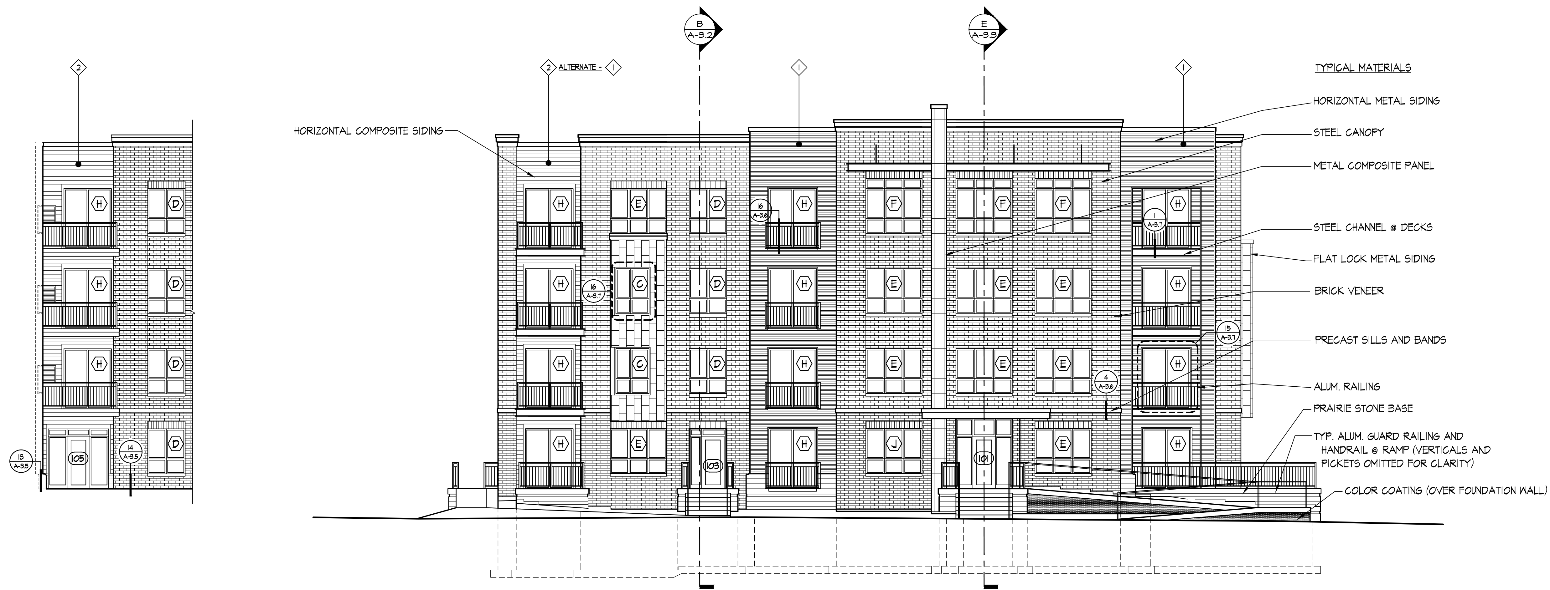
A COURTYARD ENTRY ELEVATION 1/8" = 1'-0"
