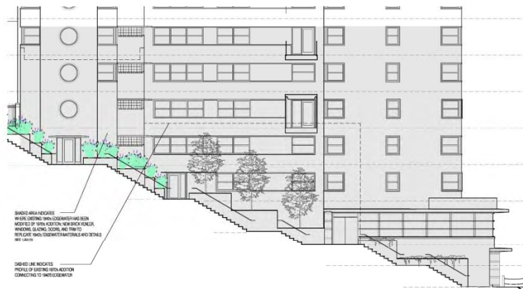
1 Partial Enlarged Elevation at New Construction SCALE: 1/8"=1'-0"
