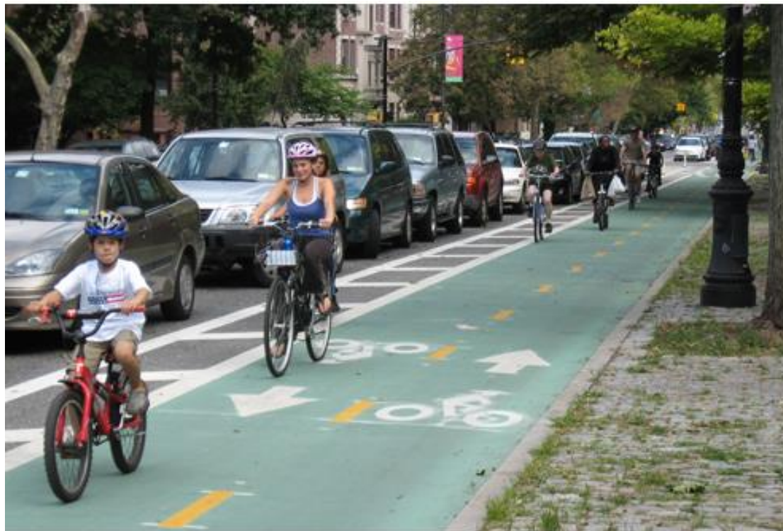
Figure B.4-10 Brooklyn, New York City – Parking protected cycletrack at street level with heavy bicycle, pedestrian and parking volumes.
