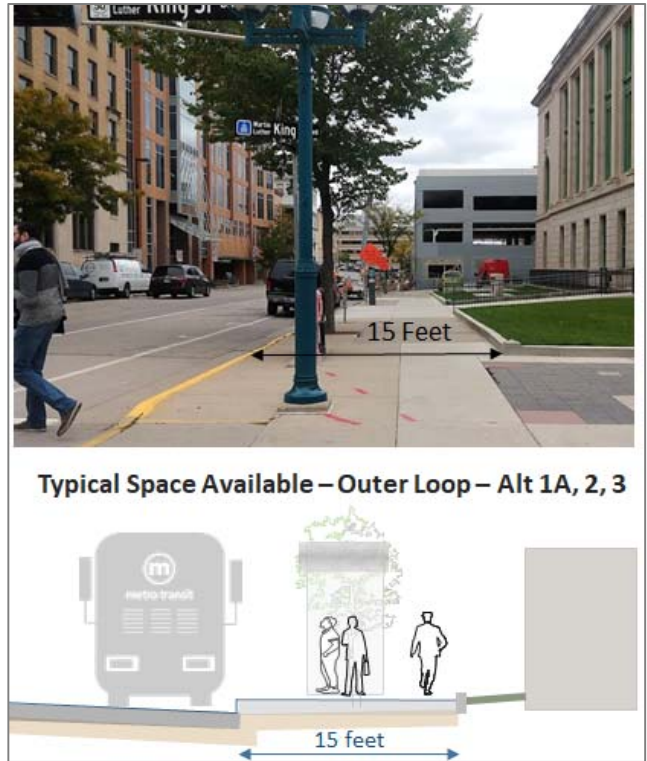
Figure 4-11 Outer Loop Doty MLK Jr Blvd BRT Station
